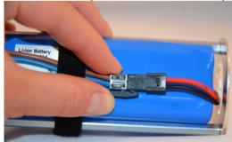
• Connect the charger connector to the battery connector. It is important that the connectors are
