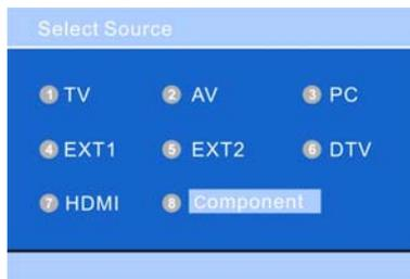
Please use numerical buttons directly to select desired signal, or use the direction to select desired signal and then press the "OK" button to confirm.
