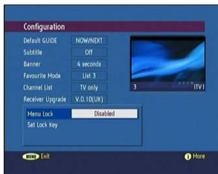
The same Parental Settings menu is used to change the PIN code. With the Set Lock Key line highlighted, press "OK" to display the Set Lock Key window. This requests the new four-digit code to be entered twice (for confirmation) and the new code comes in effect when you return to the Configuration menu by pressing Configuration menu, pressing "DTV MENU".
