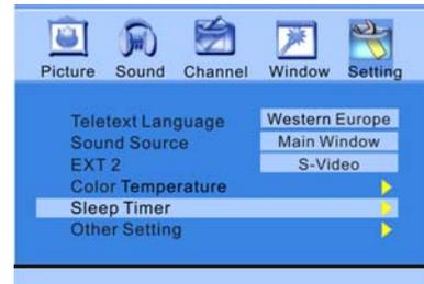
Press the " ◀/▶ " buttons repeatedly to select the duration from current to the time TV switching to standby automatically. You can select 0,10,20,30,60,90,120,180,240 minutes.
