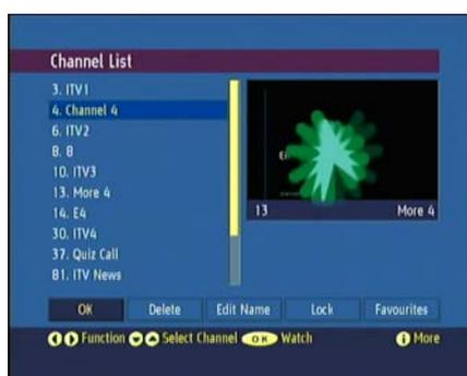
The Channel List screen displays the list of channels in the TV's memory, with a quarter-screen image window showing the selected channel, and can be used to change channels for viewing, delete channels from the memory, edit the name of the channel as it appears in the list and on-screen, lock a channel against viewing by younger members of the family, and set up favourite channels.
