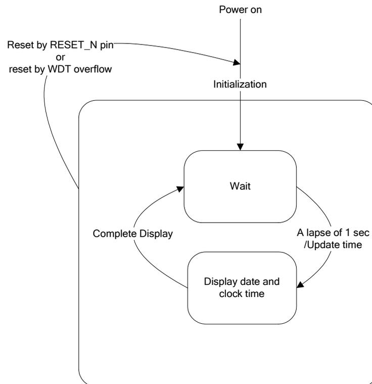
Figure 3-1 State Transition Diagram (main function)
