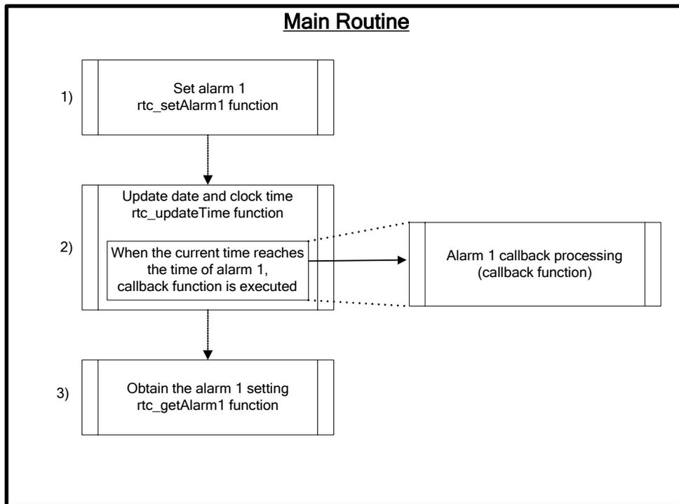
Figure 2-6 Alarm 1 Setting Procedure (Software RTC)
