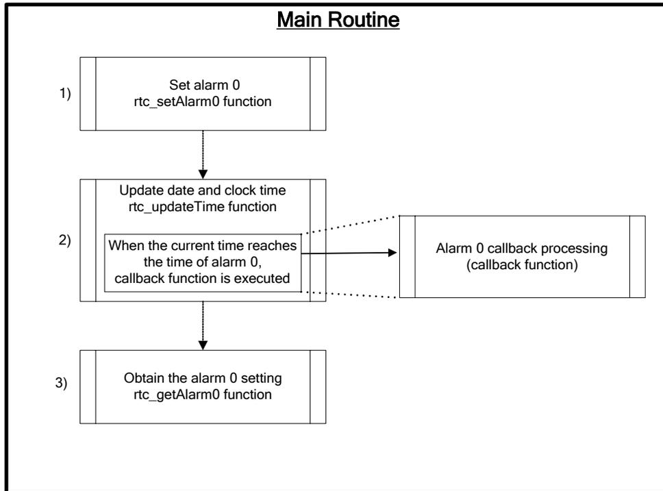
Figure 2-5 Alarm 0 Setting Procedure (Software RTC)
