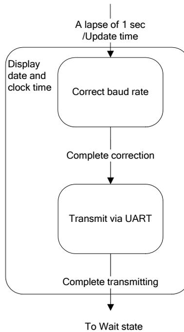
**Figure 3-2 Internal transition in “Display date and clock time” state (when use UART)**
