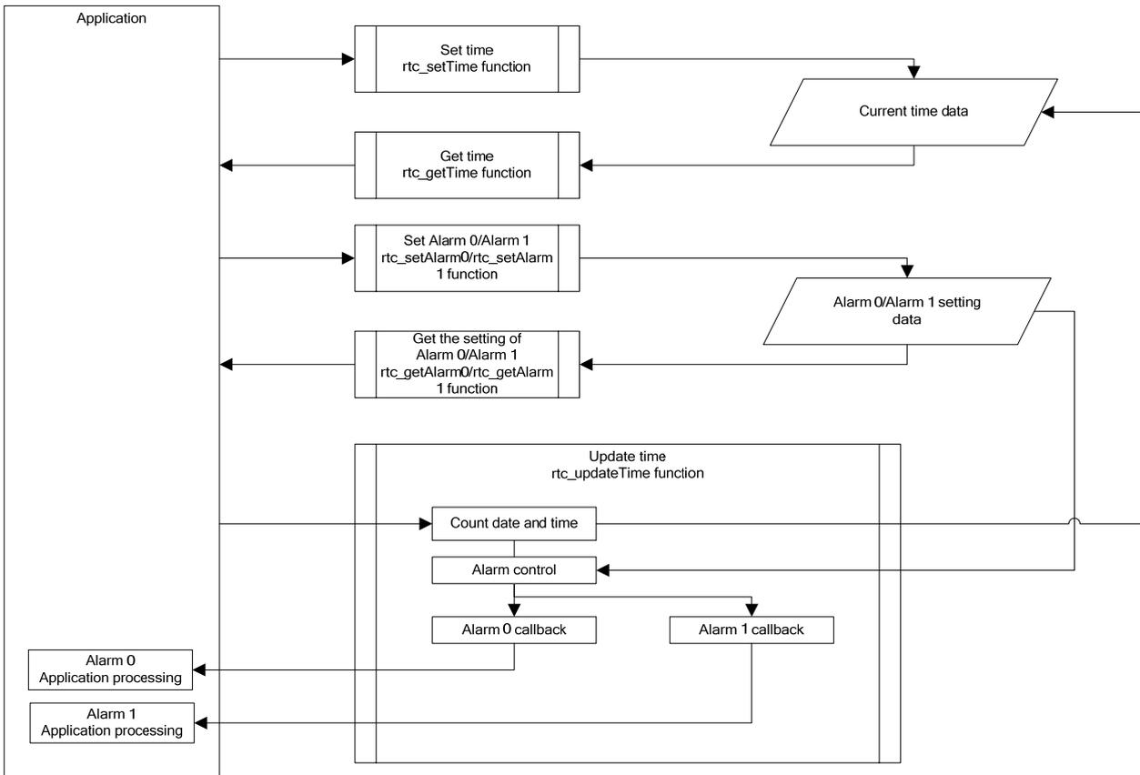
Figure 2-2 Functional block diagram of the software RTC
