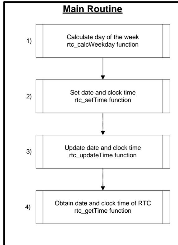
**Figure 2-4 Date and Clock Time Setting Procedure (Software RTC)**
