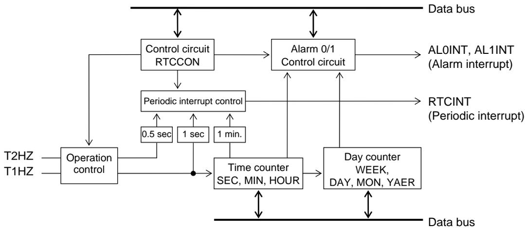
RTCCON: Real time clock control register
