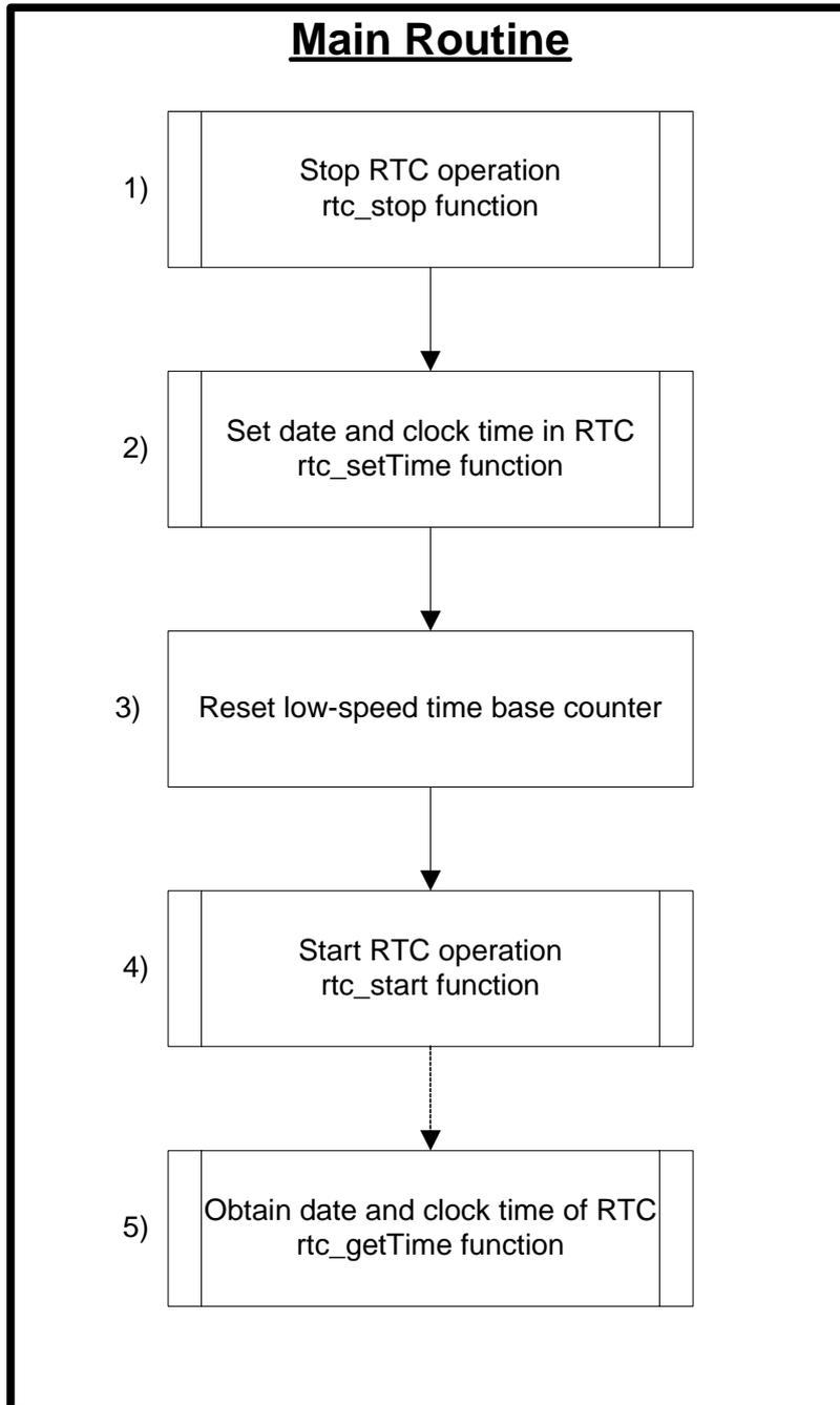
Figure 2-3 Date and Clock Time Setting Procedure (Hardware RTC)
