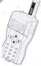
The Anilog 3060 is hand-held radio frequency identification (RFID) reader designed to simplify the recording and management of livestock identification in the field. Each animal carries a special tag which has a unique electronic identification (EID) number. The Anilog 3060 recognises this tag and can thus identify each animal. The 3060 can be used to read any international standards organisation (ISO) electronic ear tag on any animal
