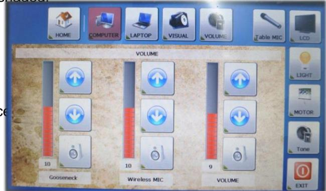
**Visual** – Selecting Visual allows you to choose from other AV equipment you have connected with the Smartium. You are also able to control basic functions equipment. After you have taught the Smartium the proper IR signals, you can turn the equipment on or off and operate basic controls for playing media.
