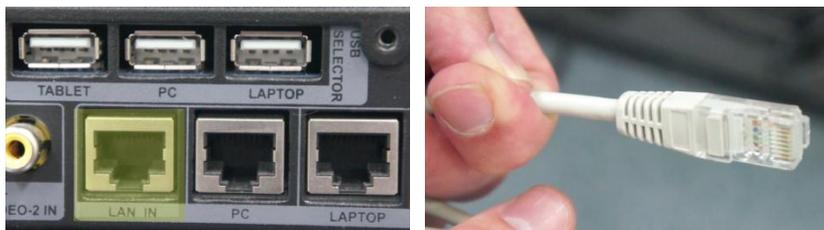
7. - If connecting the Elf to the internet or a network, you will need to connect it using an external LAN cable. The port you should connect the LAN cable to is titled LAN IN, and can be found on the back of the Controller. You can route this LAN cable into the podium by using the same hole you routed the power cable through. In the group of cables that you had originating from the controller, attach the LAN cable to your computer.
