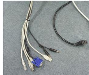
4. – You can start by connecting your mouse and keyboard to the computer. Next, in the group of cables originating from the Multimedia Controller, find the blue VGA cable. Connect it to the video out port on your computer. This cable will connect your computer to the Smartium's tablet monitor.
