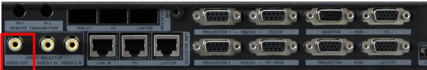
**PROJECTOR 1 / PROJECTOR 2 Control (RS232C connection)** – If the video hardware you're connecting to has an RS232C input, you can connect to this output. The RS232C cable will have 5-pins on its top and 4 on its bottom. This connection is not used for transferring video, but instead for device control. When connected, you can program the Smartium's controller to command power and other menu functions of the video display device.
