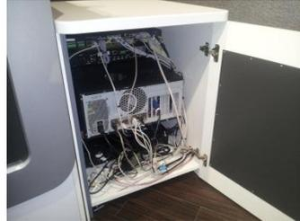
3. - Moving to the back of the Smartium, you should find a group of cables originating from the Multimedia controller and Amplifier (USB for data, USB for touch, audio, VGA, LAN). You will also find a cable to power the computer coming from the Power Adapter.
