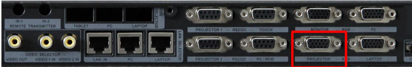
**VIDEO OUT (RCA connection)** – If the video hardware you're connecting to has a yellow RCA input, or "composite video" input as it is commonly referred, you can connect it to this output as well.
