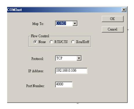
**Note1.** If any settings are changed in this part of the Virtual COM setup it will only affect the settings in the operating system Device Manager. It will not change the settings in the TRP-C38.
