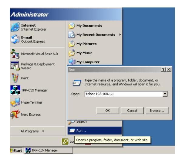
**STEP2.** Click the "OK" TRP-C38 firmware setting will show as following screen. You can set the TRP-C38 by Telnet mode.
