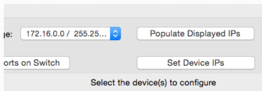
This close-up shows the "IP Range:" dropdown menu with the value "172.16.0.0 / 255.255...". Below it, the "Populate Displayed IPs" button is highlighted. Other buttons visible include "Get Device Ports on Switch" and "Set Device IPs".
