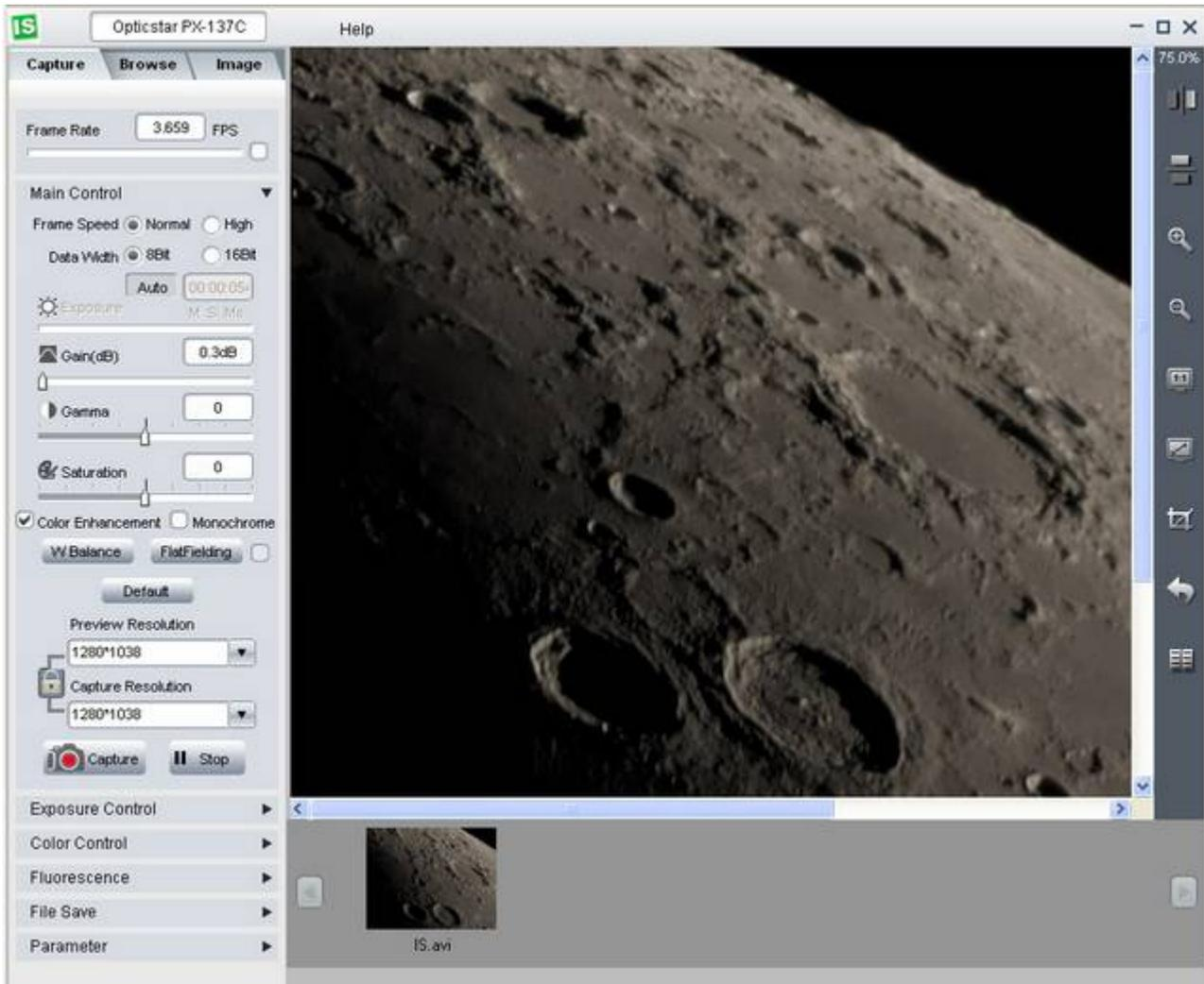
Some of the frequently used camera controls are visible on the left hand side panel of the program. Such controls include data-width and camera speed. Selecting 16-bit data width will capture higher quality images at a slower frame rate. It will also result in larger video files. Selecting high speed will result in larger video files.
