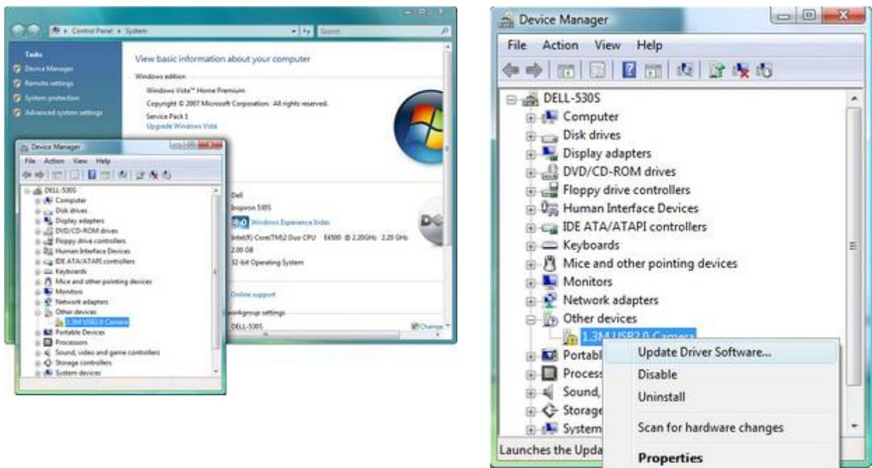
Click on the **Start** button on the Windows desktop and from **Settings > Control Panel**, select **Device Manager**. The camera should appear in the list under **Imaging devices**.
