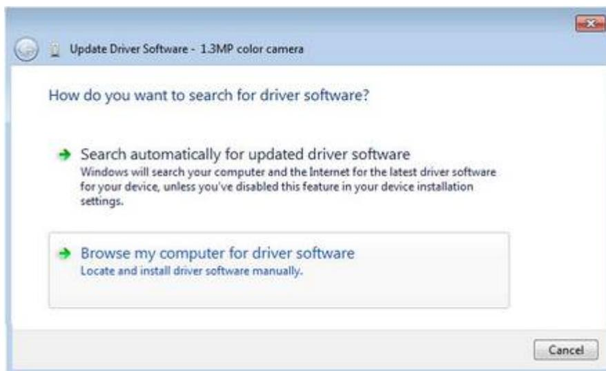
7. Navigate to the appropriate **Drivers** folder and click **Next** to proceed. For the PX-137C (colour) the drivers are situated on the CD in “\Drivers\PX-137C\64-bit” for 64-bit operating systems and in “\Drivers\PX-137C\32-bit” for 32-bit operating systems. For the PX-137M (monochrome) the drivers are situated on the CD in “\Drivers\PX-137M\64-bit” for 64-bit operating systems and in “\Drivers\PX-137M\32-bit” for 32-bit operating systems.
