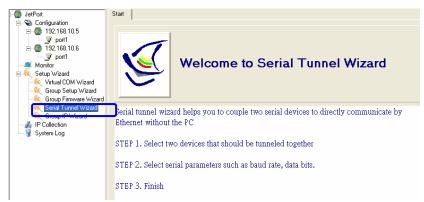
Select the devices that should be paired and move the devices into IP1 and IP2.
