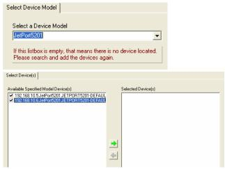
Specify the firmware image and select next. Confirm the firmware upgrade and continue operation. JetPort Commander will upgrade firmware of the devices and reboot again to finish.
