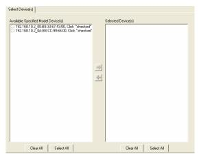
Select the devices for group IP configuration and define the IP addresses range or by DHCP.
