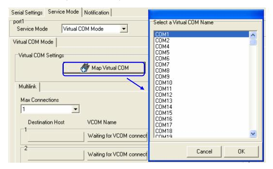
When the configuration is finished and saved, the COM port number will be shown after port, and you can monitor the port in Monitor menu.
