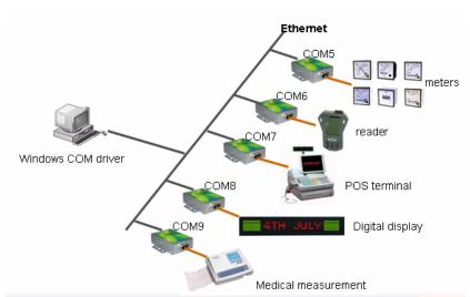
For redundant system considerations, JetPort also supports up to 5 Virtual COM links. Apply same serial setting to the backup host, all the links will transfer data simultaneously.
