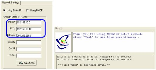
Click next to confirm the setup and the IP configuration is finished, you will see the IP addresses for the devices.
