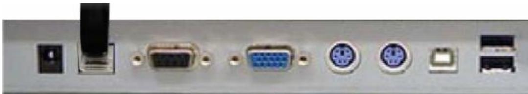
d. Connect to the COM port as shown by the picture to finish the installation
