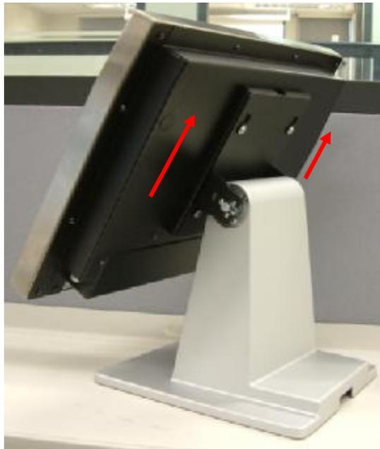
b. Lift the panel up and separate it from the stand bracket
