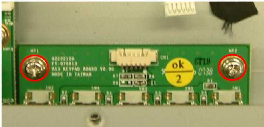
b. Remove the screws (6) to replace the OSD board
