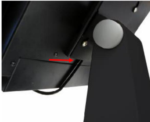
c. The cable should come out from the bottom side of the VESA bracket and band over in order to connect to the I/O port
