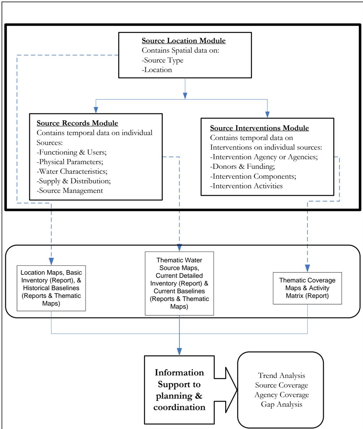
**Figure 1.1 SWIMS 2.0 Component Modules and Functionality**
