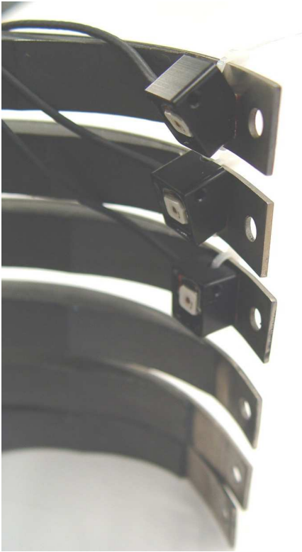
Figure 11. LEDs on Ribs #1, 2, and 3
