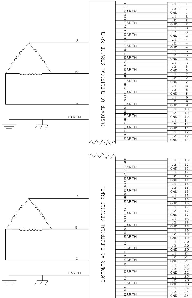
FIGURE 3-6 Δ-THREE PHASE FEED CUSTOMER WIRING (PHASE TO PHASE)
