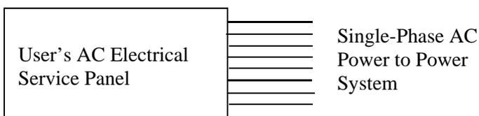
A ground is required with the AC power connections for safety and for limiting EMI/RFI emissions.
