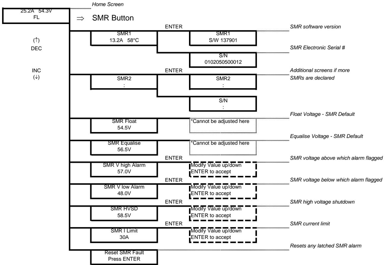
The RECTIFIER Float and Equalize voltages are the default values set in the rectifier that will be used if the Controller fails to operate. They are a copy of the raw values set in the BATTERY menu without battery temperature compensation and system drop adjustments.
