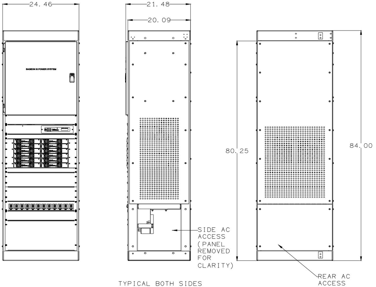
Caution: Do not block rear panel grille. A blocked grille will limit the flow of cooling air and can result in equipment overheating and failure. Minimum clearance behind and to the sides of the plant must be 2" (5 cm).
