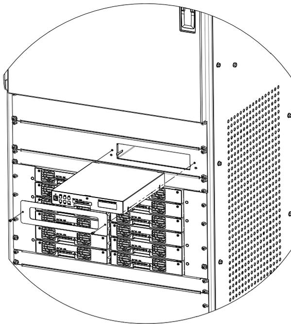
**FIGURE 6-1 REPLACING THE SCU (SAGEON III CONTROL UNIT)**
