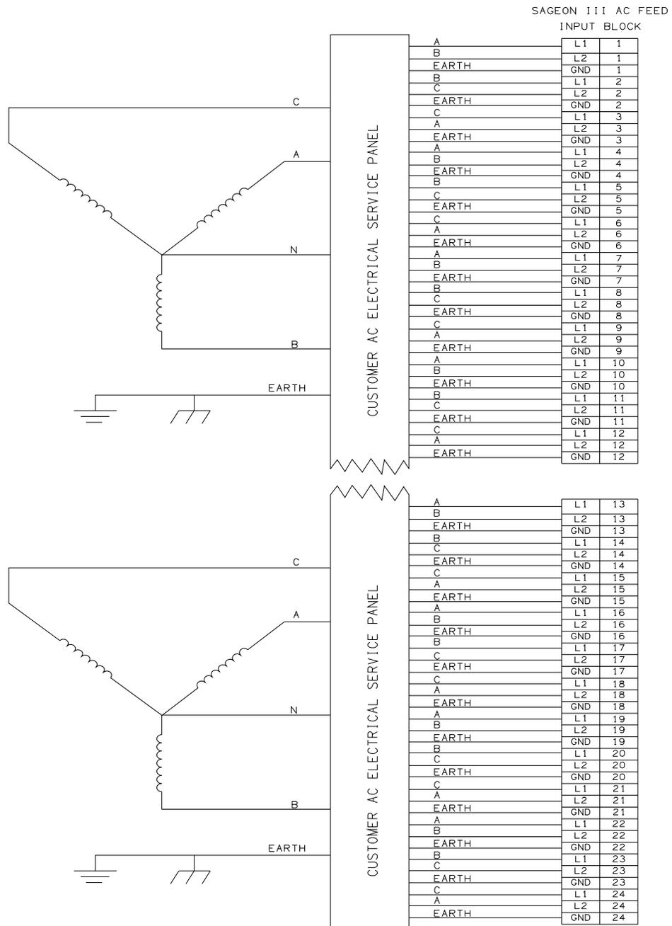
**FIGURE 3-4 Y-THREE PHASE FEED Δ-CONNECTED RECTIFIERS CUSTOMER WIRING (PHASE TO PHASE)**
