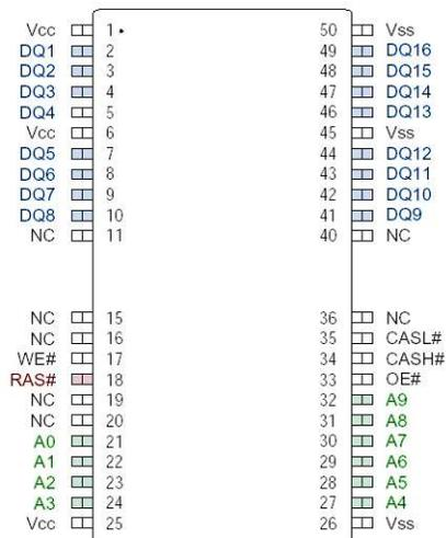
Figure: Memory Pin-Out for MK1 / MK2
