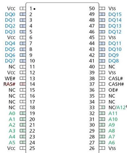
Figure: Memory Pin-Out for MK2A
