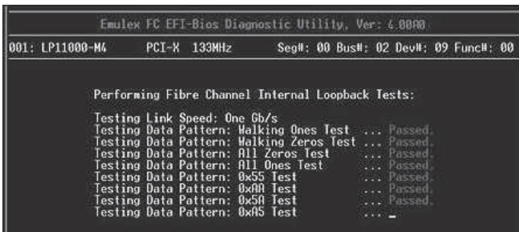
Figure 100: Internal Loopback Test progress screen
