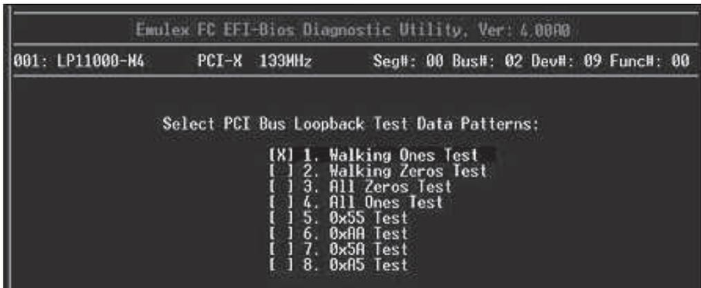
Figure 96: PCI Loopback Test Data Patterns menu
