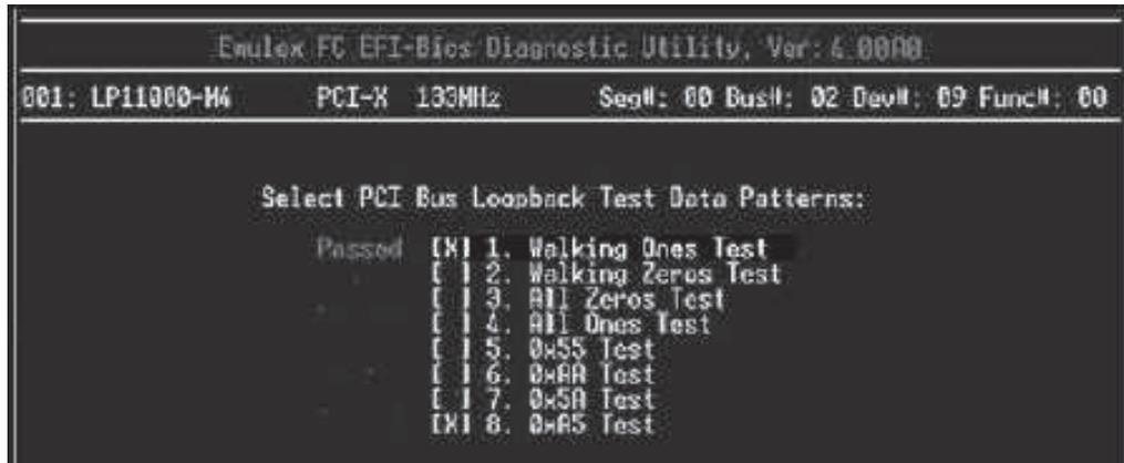
Figure 97: PCI Loopback Test Data Pattern Status menu
