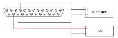
You may access MENU 6-SPECIAL TEST FUNC  $\rightarrow$  2. EXTERNAL CONTROL to choose the current monitor output range of Pin 24 at [EXTERN MONITOR] to [10 V] for 0 - 10 V (as shown in figure below) and [5V] for 0 - 5V.
