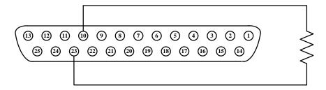
You may access MENU 6-SPECIAL TEST FUNC  $\rightarrow$  2. EXTERNAL CONTROL to choose the input resistance range at [EXTERN PROGRAM =] to [10 V / 10 K] for  $0 - 10 \text{k}\Omega$  and [5 V / 5 K] for  $0 - 5 \text{ k}\Omega$ .
