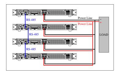
After wiring is complete, configure one of the supplies as the Master and the other three as Slave A, B, and C. After one of the supplies is configured to be the Master, it will start searching for all Slaves that are connected to the Master. To operate correctly, the user must set up the Slaves before the Master.
