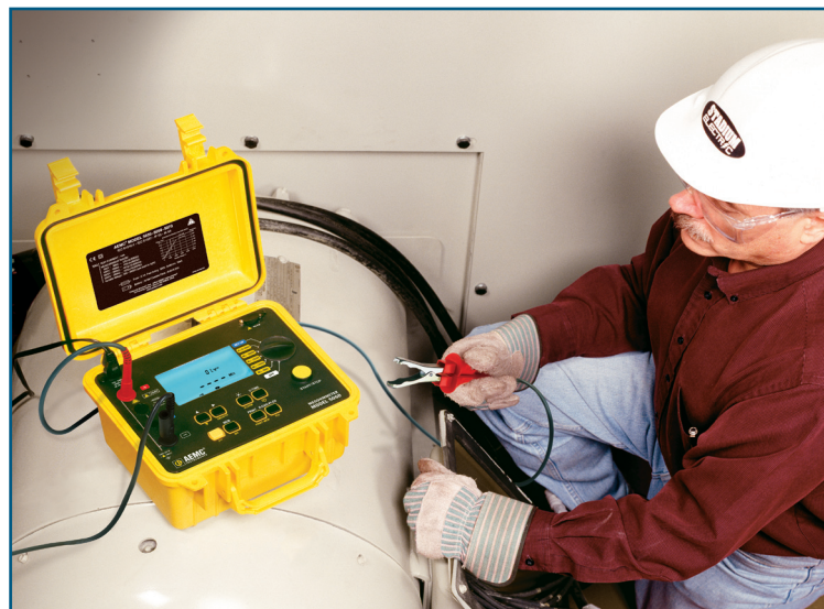
Model 5070 performing insulation test on a generator.
