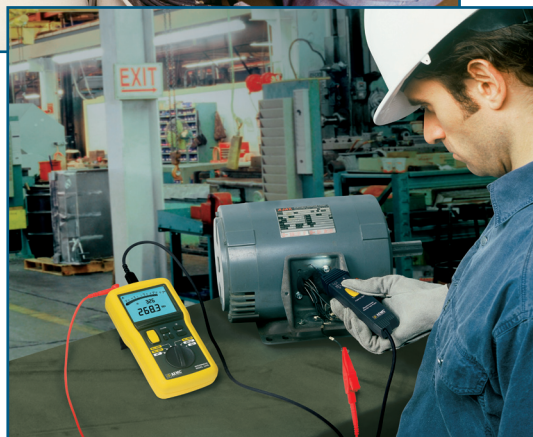
Range selection is easy to accomplish with the large positive action rotary switch on the front panel.
