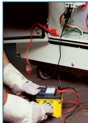
Model 1250N performing a hand-cranked 1000V test on a generator.
