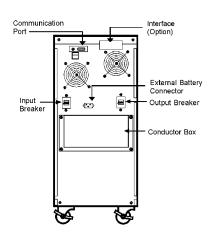
Figure 1 MCP 6KVA
