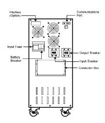
Figure 2 MCP 10KVA
