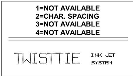
Place the unit in the Command mode and press **F1**. The screen shown to the left is produced. Press the correct number to make changes to that parameter. Those selections designated as NOT AVAILABLE will not respond to selection. They are reserved for future system expansion.
