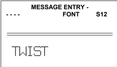
Enter the Message Entry mode by pressing . The top portion of the screen will change as shown on the left. The default font style is S12 (12 x 9 character) for all TTP Models. If a different font is desired, press until the desired font is shown. The font shown is the one used in building the message from this point on.
