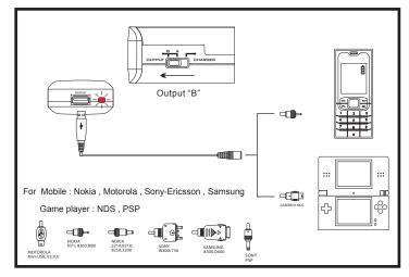
4) After fully charged the selected devices, unplug the cables and switch the button back to the "Charger" position. RED LED light will turn off immediately and the output process will be stopped. For safety renson, please take off the batteries form the C-515 charger after used.
