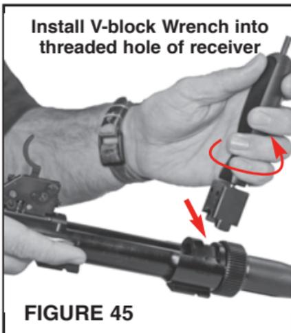
Use Hole Marked "L" to loosen barrel nut
