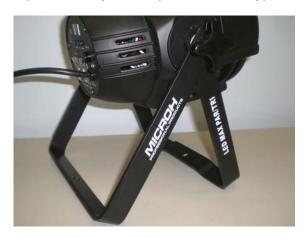
Clamp Mounting: The MICROH LEDPRO64RGBW provides a unique mounting bracket assembly that integrates 2 brackets to be used to mount on a truss or the floor. When mounting this fixture to truss, be sure to secure an appropriately rated clamp to the included bracket fitted through the center hole. As an added safety measure, be sure to attach at least one properly rated safety cable to the fixture.
