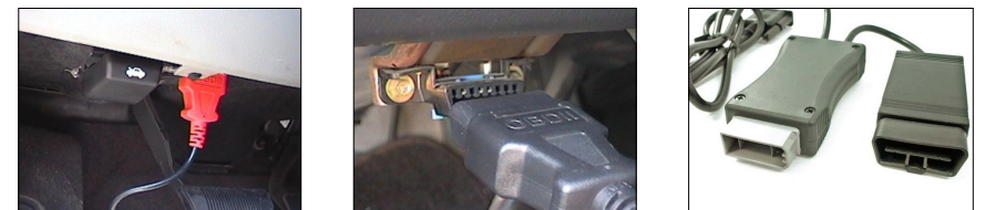
Red OBD II connector - Grey OBD II Connector - Nissan OBD I & OBD II
