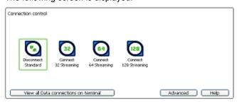
b. Select the required streaming connection, for example **64 Streaming**. The following message is displayed, asking you to confirm that you want to close your current connection and open a new connection, charged by time:
