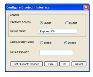
b. If the Bluetooth interface is not enabled, check **Enable**.
