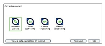
If the standard connection is open, the words **Disconnect Standard** are displayed below the connection icon.
