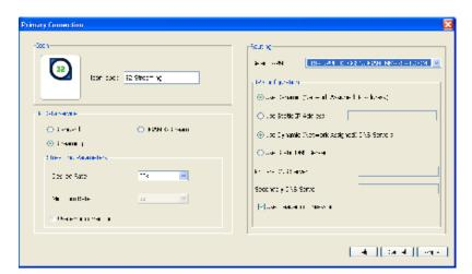
b. Verify the APN displayed in the **Select APN** field. If it is not correct, select the required APN from the drop-down list and click on **OK**.
