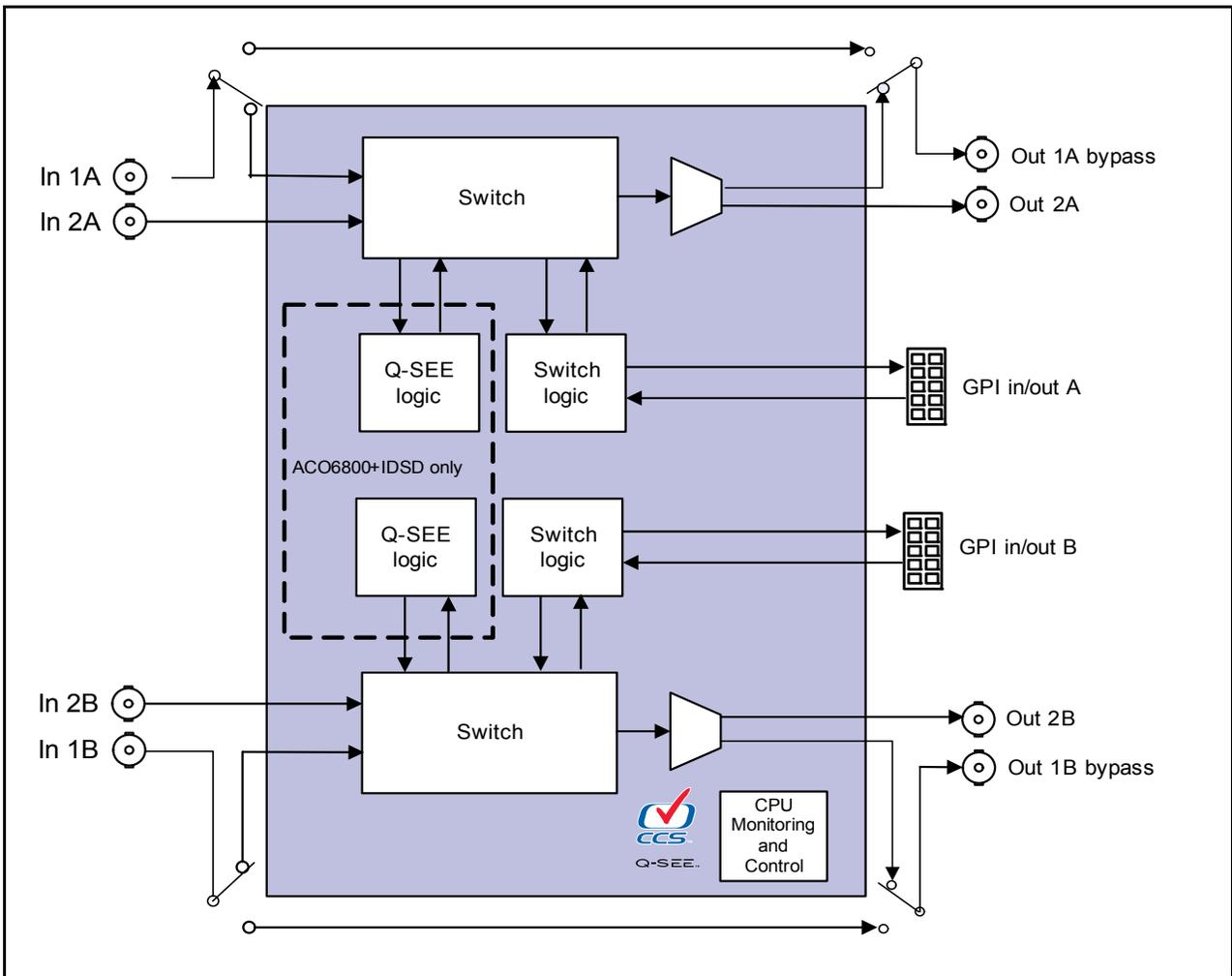
**Figure 1-6.** Signal Flow Diagram for ACO6800+DSD and ACO6800+IDSD
