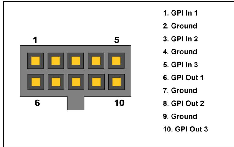
**Figure 1-3.** GPI Connector Pinouts
