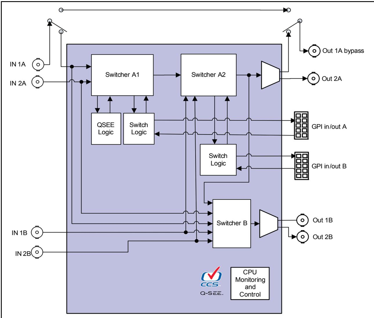
**Figure 1-4.** Signal Flow Diagram for ACO6800+4X2D
