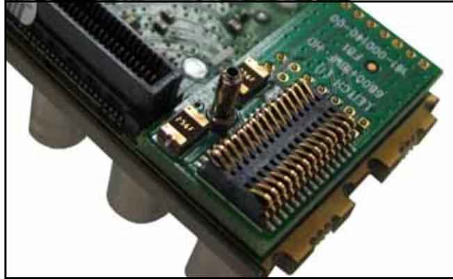
**Figure A-1.** Typical Back Module Spring Connector
