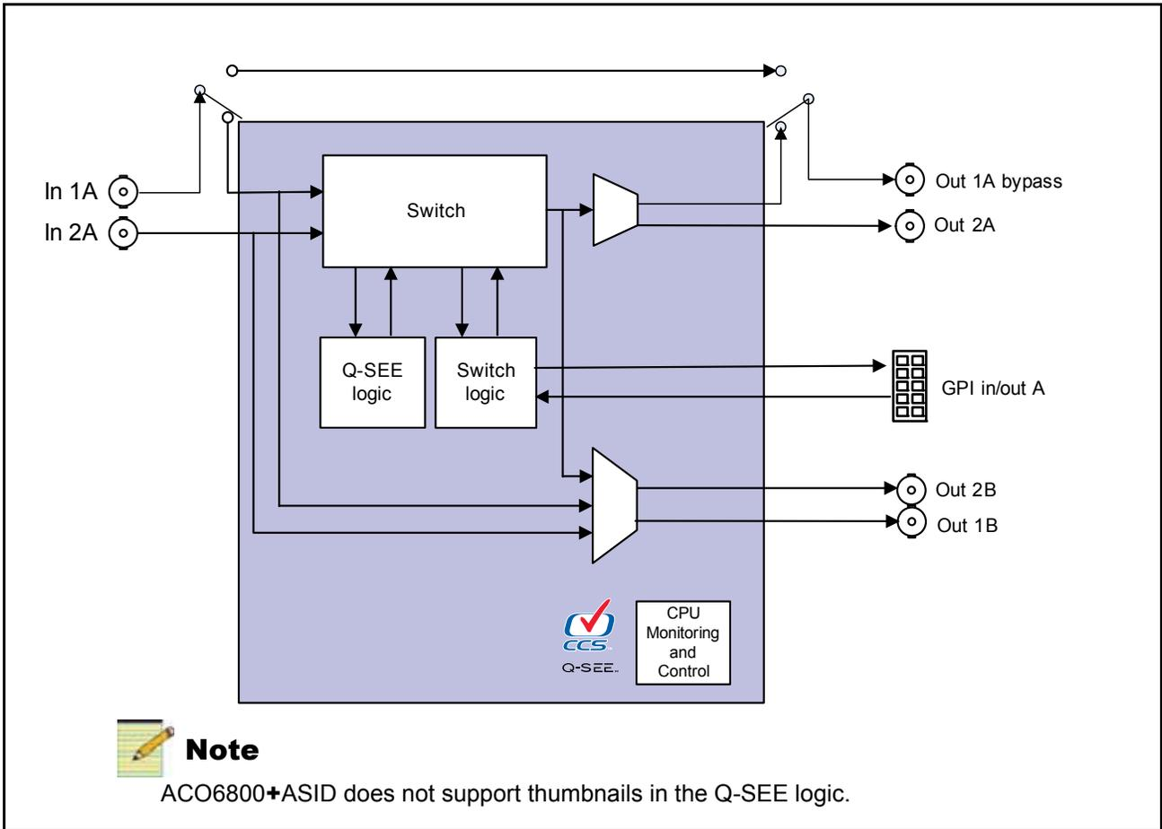
Figure 1-5. Signal Flow Diagram for ACO6800+ASID and ACO6800+ISD
