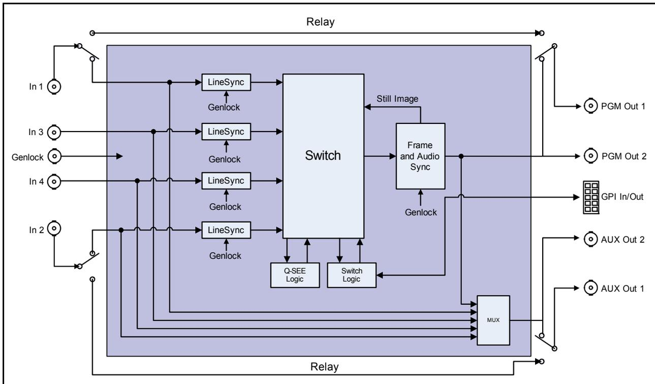
**Figure 1-7.** Signal Flow for ACO6800+4X2+ICQST
