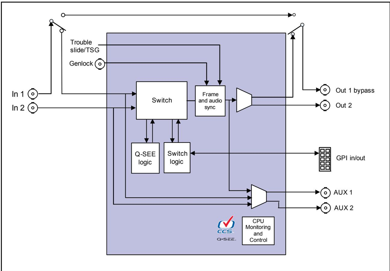
Figure 1-8. Signal Flow Diagram for ACO6800+ISCST
