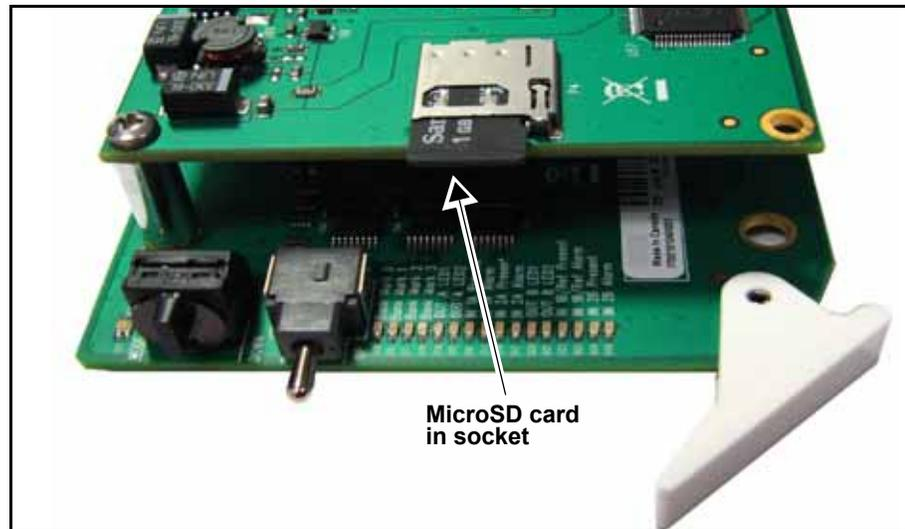
**Figure 2-6.** Inserting the MicroSD Card
