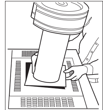
Figure 5. Vent cap with adapter plate (outdoor).
