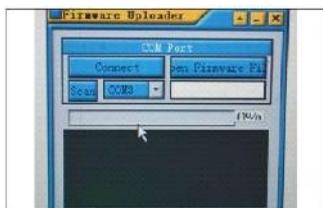
3. Open the latest firmware upgrade program, available from <http://www.freexgroup.com/downloads.php>. Select the correct COM Port. Check with your device manager to find out the correct port used by the USB dongle.
