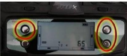
Press Menu again to move the slider to Channel 1, 2 or 4 and use "+" or "-" buttons to change values to your desired values. Normally 65% is a good value for beginners. It makes Quadcopter very docile and easy to control.
