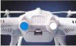
**Compass Calibration:** During compass calibration, left LED will turn solid Blue. That means compass is open for Calibration. After calibration, you can turn the compass calibration off and Blue light will turn off. Also during this process, blue light will turn on when the compass points to magnetic north and will turn off when compass is not pointing to magnetic north. This provides a very simple way to detect magnetic north and do the compass
