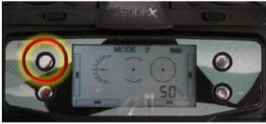
Press and hold the menu button and power on the radio.
