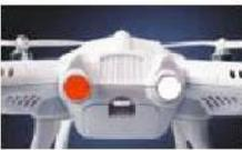
**Control Signals:** If the left LED is Solid Red, that shows the binding process. Once successful bound with radio, the Red LED will go off.
