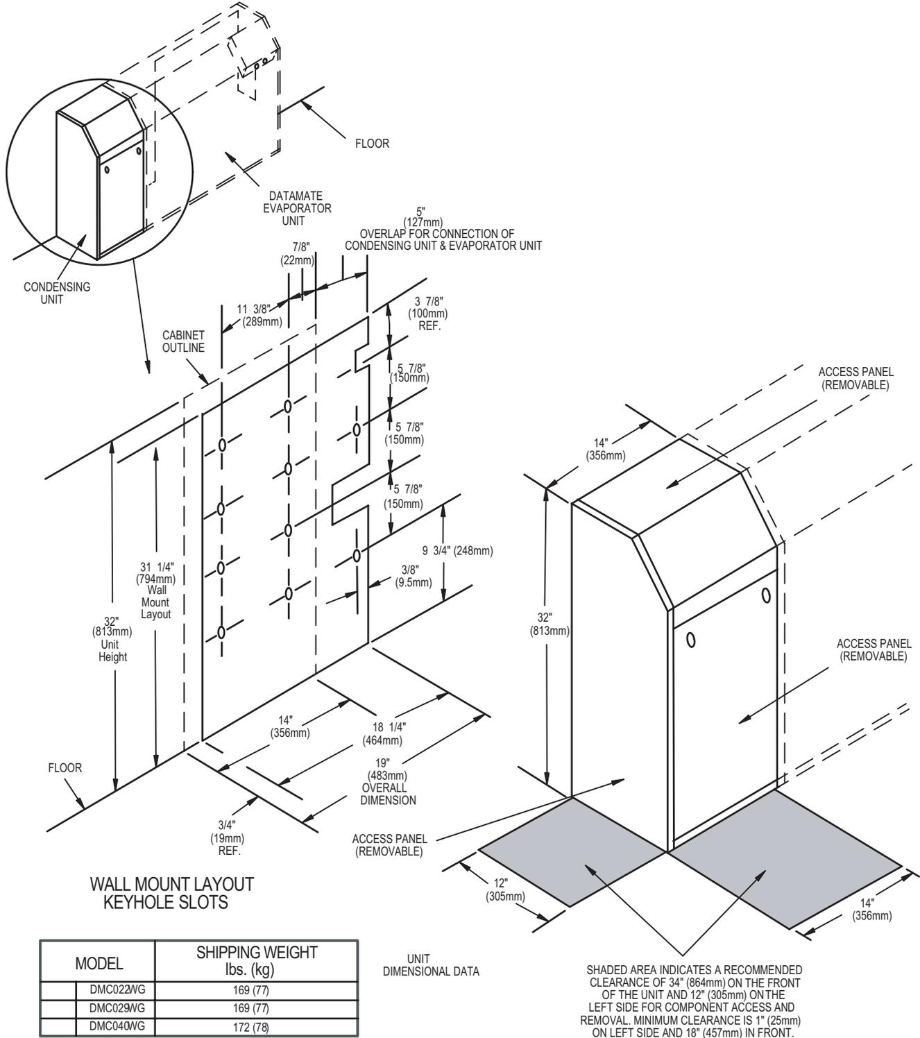
Unlatch the front cabinet door and remove the two screws that secure the cabinet to the chassis. Lift off the cabinet. Eight keyhole slots are provided for mounting the unit on the wall (refer to **Figure 17**).
