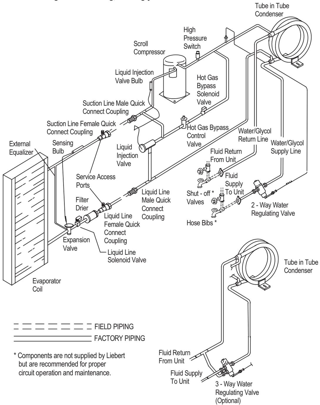
Figure 14 General arrangement drawing, air cooled
