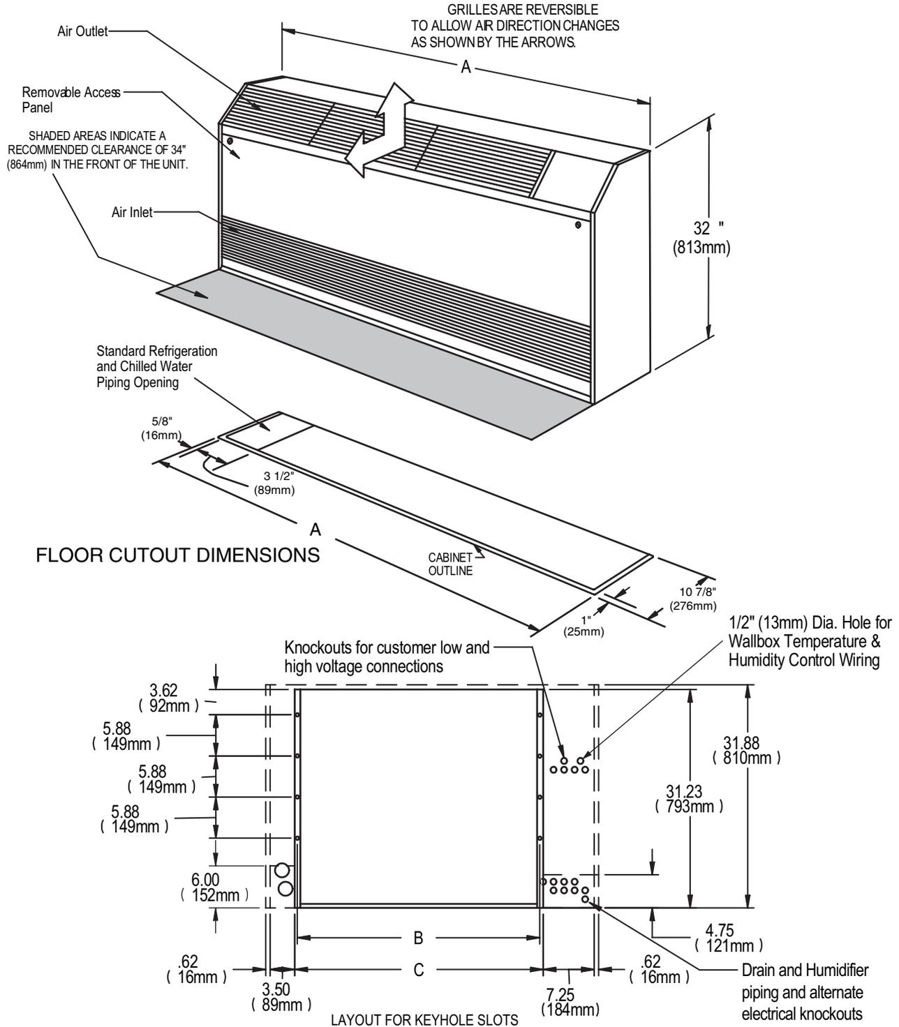
**Table 5 Fan/coil and chilled water module dimensional data**
