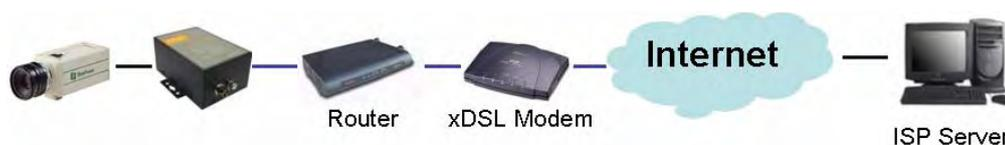
In this case, a router with PPPoE is required to dial up to the ISP and the IP address must be fixed to retain the video server's network connection.
