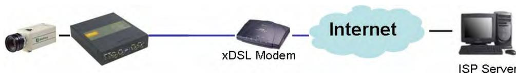
The VPort 2141 with PPPoE function can dial up to an ISP automatically, and the IP address is not necessary to be fixed, since a startup log will be sent to the administrator by email or FTP (SMTP and FTP server must be setup) to notify the current IP address once it has been changed by the ISP server. This method is more cost-effective than applying for a fixed IP address.
