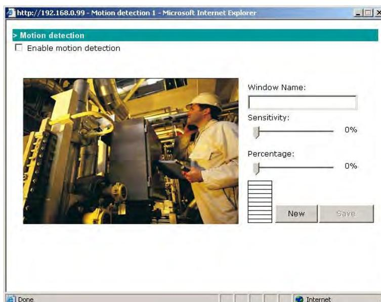
Three areas of the image can be configured for the VMD (video motion detection) function. The VMD alarm will only be triggered when the VMD conditions in these 3 specific areas are met. Each area can be fine tuned to fit the environment for different VMD conditions by setting the **Sensitivity** and image change **Percentage**.
