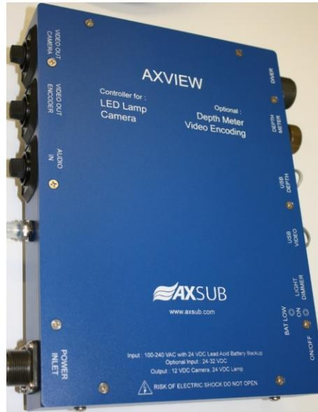
On the top side of the AxVIEW, there are 4 screws to install a bracket to fix the product on a wall or in a cabinet to liberate space on the working surface. Do not remove feet under the unit. There are up to 4 connectors on the left side of the unit:
