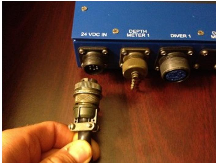
1. Connect the Depthmeter Cable (if equipped) on the 4 pins AMPHENOL connector. If the SMART Camera is used, you do not need to install this cable.
