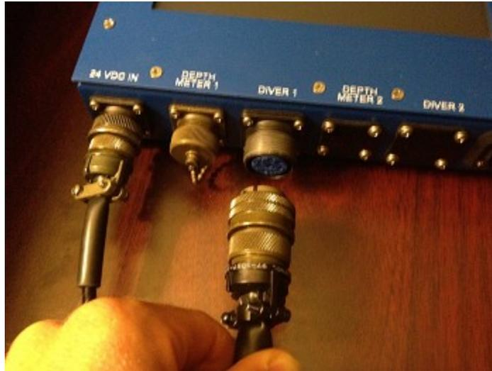
3. Connect the Camera, the Lamp and the Depthmeter (if required)
