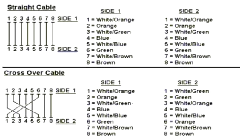
Figure A-1: Straight-Through and Crossover Cable
