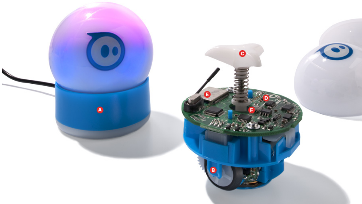
Figure 3.1 shows the inside of Sphero and the assembled Sphero in its charging dock. Permission Pending.
