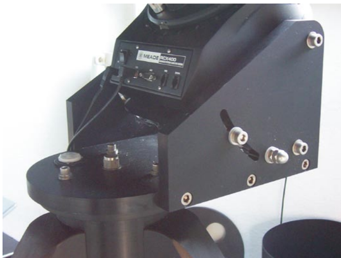
Fig. 4.1 Telescope mounted on an equatorial wedge, showing side bolts and latitude adjustment slot
