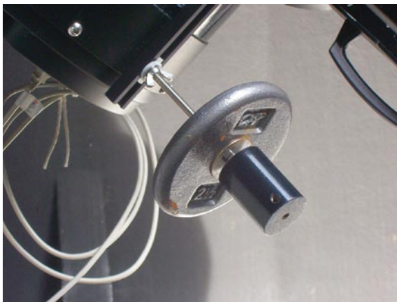
Fig. 4.5 The additional balance weight required when adding a guide ‘scope
