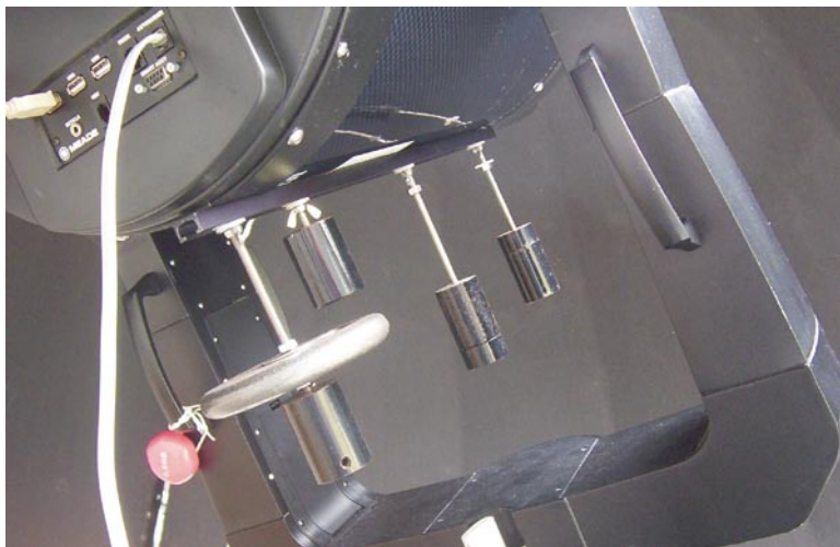
Fig. 4.4 Rear of LX400 showing rail fitting with various weights on different rod lengths
