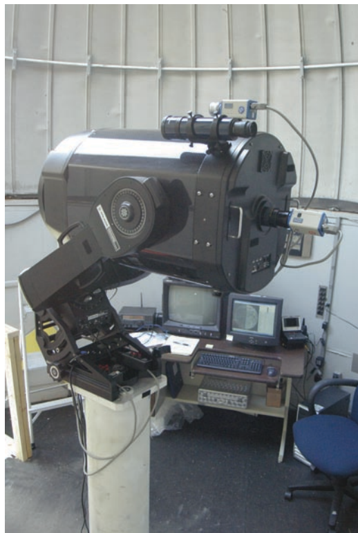
Fig. 11.1 A 14 in. (35 cm) LX400 telescope with a focal reducer and astronomical video cameras at the Automated Lunar and Meteor Observatory (ALaMO). This telescope is used to observe the Moon for lunar impact flashes (NASA) (Images credit Science@NASA)
