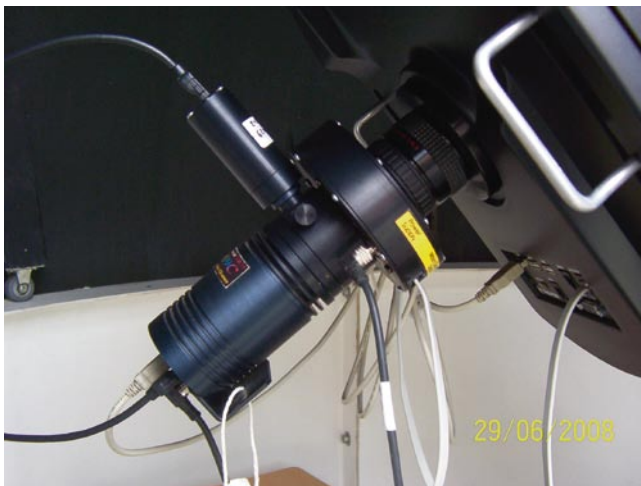
Fig. 9.3 Starlight Xpress Adaptive Optics unit fitted to telescope. Additional cables are used to control the tilt plate
