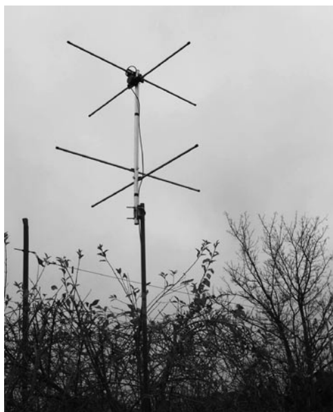
Fig. 10.7 Crossed dipole antenna for weather satellite reception. This is conveniently lightweight and easy to fit to a mast
