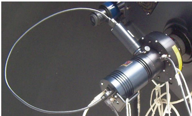
Fig. 3.5 A Starlight Xpress adaptive optics unit fitted on the LX400 telescope. Note the need for extra control cables
