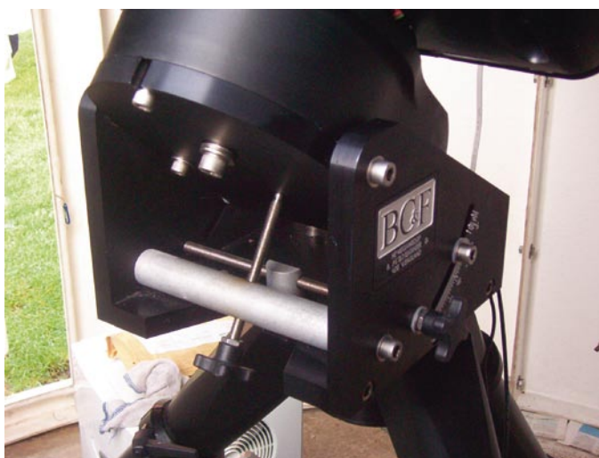
Fig. 4.2 Rear of wedge (the view from the south side) showing a latitude adjustment bolt
