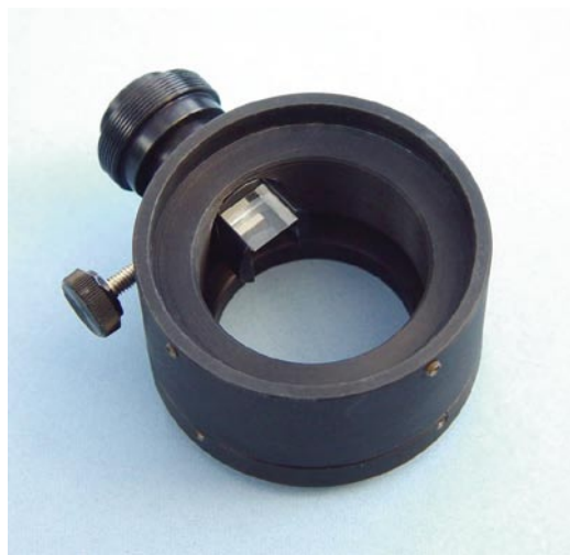
Fig. 9.4 Off-axis-guider (AOG) assembly showing sampling prism
