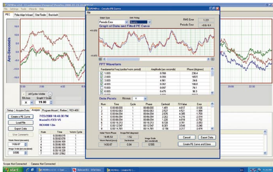
Fig. 6.8 PEMPro analysis of raw periodic error. The best fit curve can then be selected
