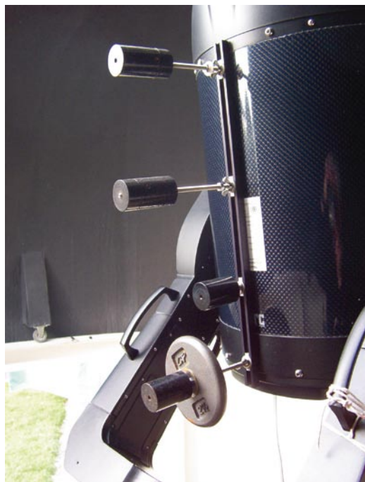
Fig. 4.6 Balancing the LX400 OTA in vertical position
