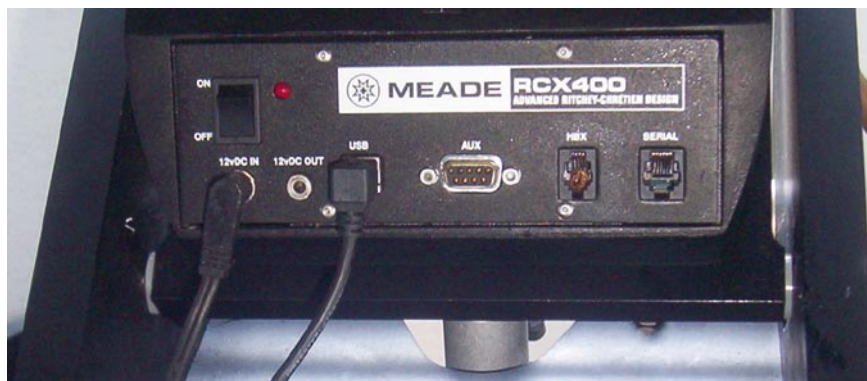
Fig. 2.5 Front panel of the LX400 telescope. Connectors left to right are for USB, auxiliary connection ( see text ), main handbox, and a serial connector
