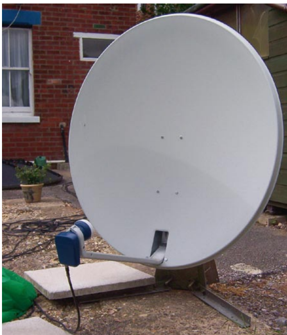
Fig. 10.9 EumetCast DVB reception equipment for Europe's MSG-2 imagery broadcast from the HotBird satellite
