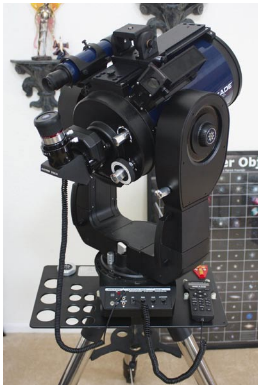
Fig. 2.11 Jim West's customized LX200 showing an eyepiece tray and Telrad finder
