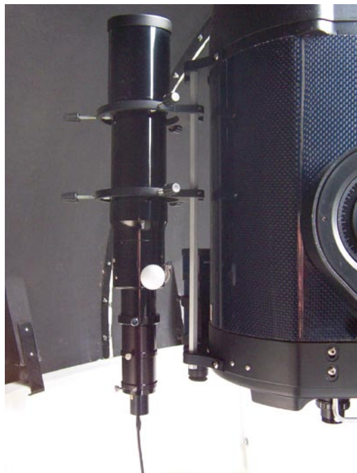
Fig. 4.7 A heavy guide ‘scope requires extra balance weights
