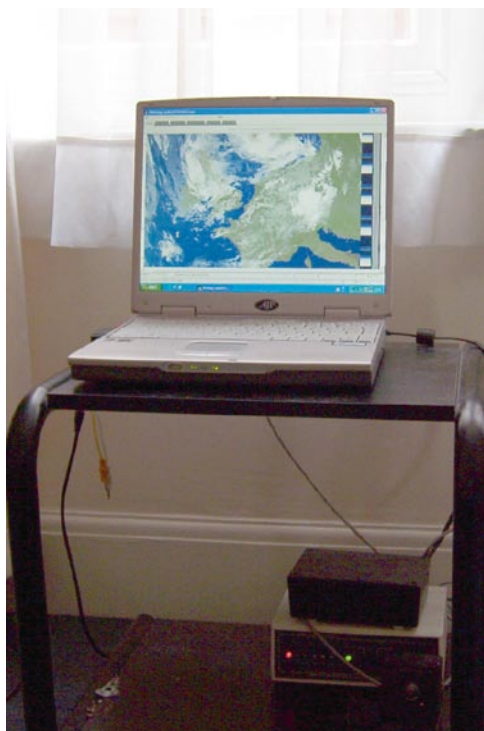
Fig. 10.8 A dedicated laptop receiving a.p.t. from a nearby external antenna. The laptop does not require a high specification
