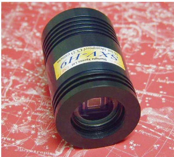
Fig. 3.3 Starlight Xpress SXV-H9C one-shot color camera. This can be used for deep sky imaging as well as astrometry
