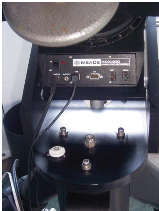
Fig. 4.3 Upper face of wedge showing bubble level and bolts securing wedge to mount
