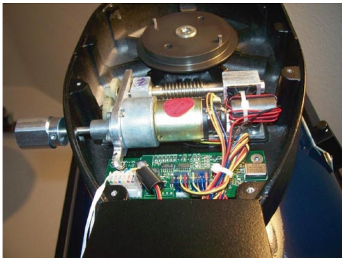
Fig. 6.1 The declination motor on the west fork arm of an LX200GPS seen with cover off (Courtesy of Robert Kessler)
