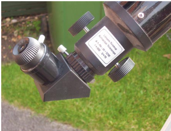
Fig. 1.3 The accessories that come with a small telescope usually include a right-angled prism. This enables the astronomer to view the heavens in a comfortable position rather than getting a cricked neck
