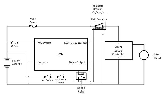
In some golf cars, the foot pedal controls the main contactor. The foot pedal is connected directly to the key switch and this point is not easy to get to. A relay can be added as shown to control the signal from the foot pedal.
