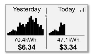
The graphs show hourly data, with a bar for each hour. The height of the bars is proportional to the number of kWh consumed for each hour. The graphs are autoscaling, and meant to show relative, rather than absolute values. The small number near the top of the center line indicates the value (in kWh) of the highest bar in the graphs.
