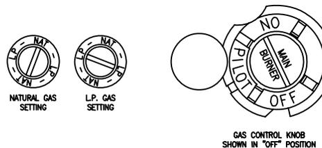
3. Change the pilot regulator by removing pilot regulator cap. Depress and rotate knob counterclockwise
