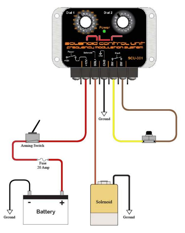
**IMPORTANT**—the SOL+ output is internally over current protected and MAY turn OFF without warning. Always test before use to determine that an over current condition does NOT exist!
