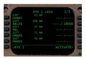
A second example of the PB/PB in practical application comes from defining points along an approach path. If, for example, an approach or STAR has an altitude restriction that is based upon the intersection of a VOR radial across your path of flight, you can use a PB/PB waypoint to make the point appear visually on your flight plan along with the associated speed/altitude restriction.
