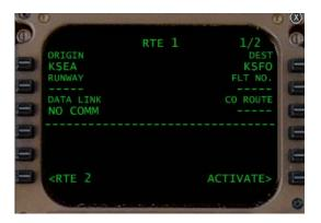
CO ROUTE: If a company route was previously stored for this flight, entry of the stored route name into line 3R via the scratchpad will automatically load the flight plan. This will eliminate the need to enter ORIG and DEST, as well as eliminate the need to program the route of flight in the RTE LEGS pages.
