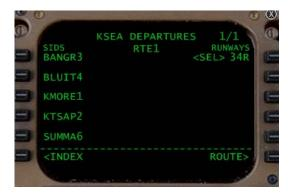
Standard Instrument Departures: The SIDS are listed on the left side of the display at 1L through 5L. A SID can be selected by pressing the associated LSK. Once a SID is selected, a <SEL> indicator will appear next to the associated SID to indicate that it has been selected.
