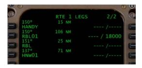
PBD bearing entries from 0 to 360 degrees and distance entries from 0 to 700 miles are valid.
