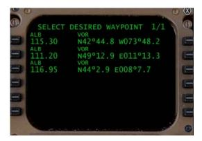
The VORs are ordered by distance from the fix prior to the entry selection, or the airplane's current position if no fixes have been entered. Pressing a left side LSK will select the desired item into the flight plan automatically.
