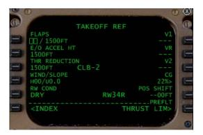
Flap Setting/Flap Acceleration Height: The planned flap setting (flaps 10 or flaps 20)
