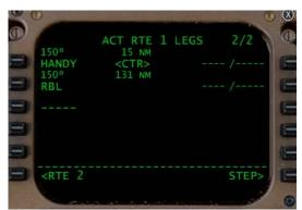
At the bottom of the LEGS display, the <RTE 2 LEGS prompt allows the crew to display RTE 2 legs and waypoints if a RTE 2 has been programmed.
