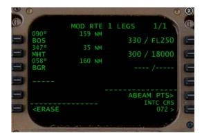
Pressing the EXEC key will confirm the change, or pressing <ERASE will cancel the Direct-To selection. Once the <EXEC key has been pressed, the FMS will be updated to fly Direct-To the desired fix.
