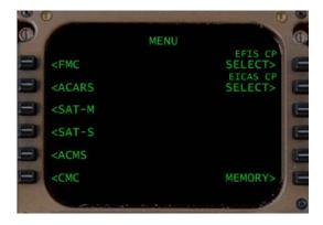
Pressing the LSK 1L key, (the <FMC prompt) will enter the FMC function area and display the IDENT page, as follows:
