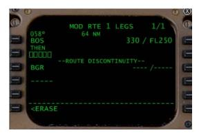
To confirm the continuation of the route, the waypoint identifier for the next fix in the desired route sequence should be downselected to the scratchpad by pressing the associated LSK.
