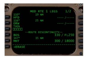
In order to continue navigating normally, the route discontinuity must be removed by telling the FMC which fix is to follow the newly added fix.
