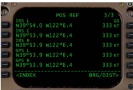
Page 2/3 FMC POS: Line 1L displays the current FMC computed aircraft position and the source of it's current position data. In the event the position update capability of the FMC fails or is inhibited, this line will be blanked by the FMC.
