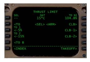
The THRUST LIM page displays three takeoff thrust limit options at lines 2L through 4L. Lines 2R through 4R display climb thrust limit options.
