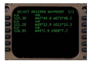
All navigation aids with names identical to that entered in the FMC scratchpad will be displayed. In some cases, the crew member may need to use the NEXT PAGE/PREV PAGE keys to page through multiple displays in order to locate the desired fix.
