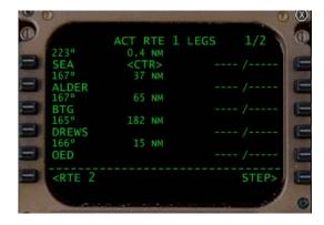
The Title line of the page describes which route is currently being displayed on the RTE LEGS page. The upper right hand corner shows which page of the LEGS display is currently being shown. The NEXT PAGE and PREV PAGE keys are used to scan forward and back. Page 2/2 appears as:
