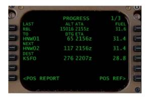
LAST / ALT: Line 1L displays the identifier of the last navigation fix most recently overflown. This line will be blank if there is no active flight plan programmed, the first leg is still being flown, or after flight completion. The ALT indicator in the center of line 1 shows the airplane altitude at the time of fix crossing.
