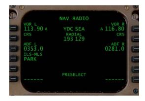
The NAV RAD page is allows the crew to monitor auto-tuning activity, or to manually tune a desired frequency for VOR1/VOR2, ADF1/ADF2 or the ILS.
