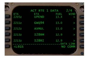
The RTE DATA page is divided in to four columns. The entire remaining portion of the flight plan can be paged through using the NEXT PAGE / PREV PAGE keys on the FMC/MCDU keypad.
