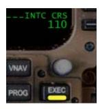
In the current example, our flight has been instructed to fly a heading of 150 until intercepting the 290 radial. As such, we enter the inbound course of 110 degrees (290-180 = 110 on the inbound course!)
