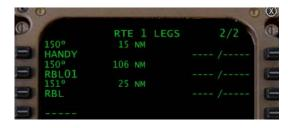
The along track waypoint that has been created is now listed in the flight plan using the format PPPss, where PPP is the first three letters of the fix name upon which the custom waypoint is based, and ss is a sequence number assigned by the FMC.
