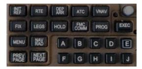
**MENU Key:** The MENU key provides access to the FMC and other aircraft subsystems which use the CDU for input or control. When pressed, the MENU key brings up the following display screen on the CDU:
