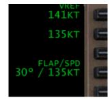
Additionally, the crew may manually enter a desired flap setting/Vref speed by entering the information into the scratchpad in the format FF/SSS.
