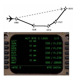
A Direct-To routing is performed by displaying the ACT RTE LEGS page or the MOD RTE LEGS page, then entering the desired fix into the scratchpad. This can be done by manual entry, or be down-selecting the fix from the displayed flight plan.
