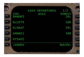
Runway: The available departure runways for the selected airport are listed down the right side of the screen. Pressing an associated LSK will cause all other runways to be removed from the screen and a <SEL> indicator will be placed next to the selected runway to indicate that it has been selected as the departure runway.
