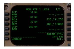
Once the desired station has been entered into the scratchpad, it should be up-selected to 1L in the ATC RTE LEGS page.
