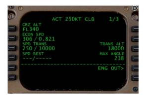
CRZ ALT: The cruise altitude is displayed at 1L with the header of CRZ ALT. The current cruise altitude is displayed if one has been selected and CLB is the active mode. If the current altitude is not displayed, 1L will contain prompt boxes which can be replaced by up-selecting the desired cruise altitude from the scratchpad.
