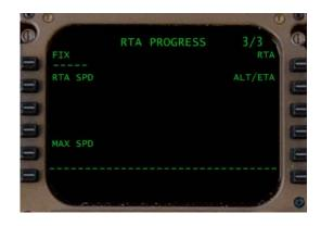
**PROG Key:** The PROG key accesses the flight PROGRESS pages. These pages provide navigation fix, distance to go, fuel,
