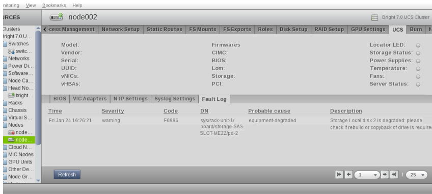
Figure 5.9: CIMC Fault Logs In cmgui
