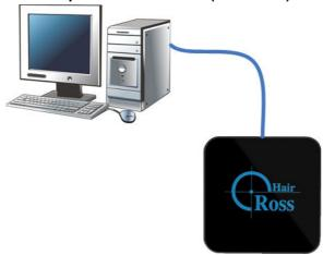
• Please connect your Cross Hair according to the figure above, using the USB cable included in the package. **Make sure that there is no controller, keyboard, mouse, joystick or anything else plugged into it.** And when Cross Hair LOGO is white, it enters into **PC MODE**, and can then be configured on PC.
