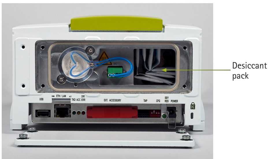
Figure 25. Replacing the desiccant
