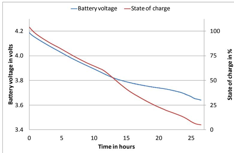
*Figure 56: Typical discharging characteristics of extended LiPo battery*
