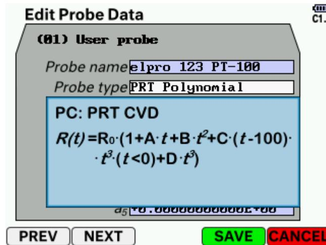
Figure 29: Probe type selection
