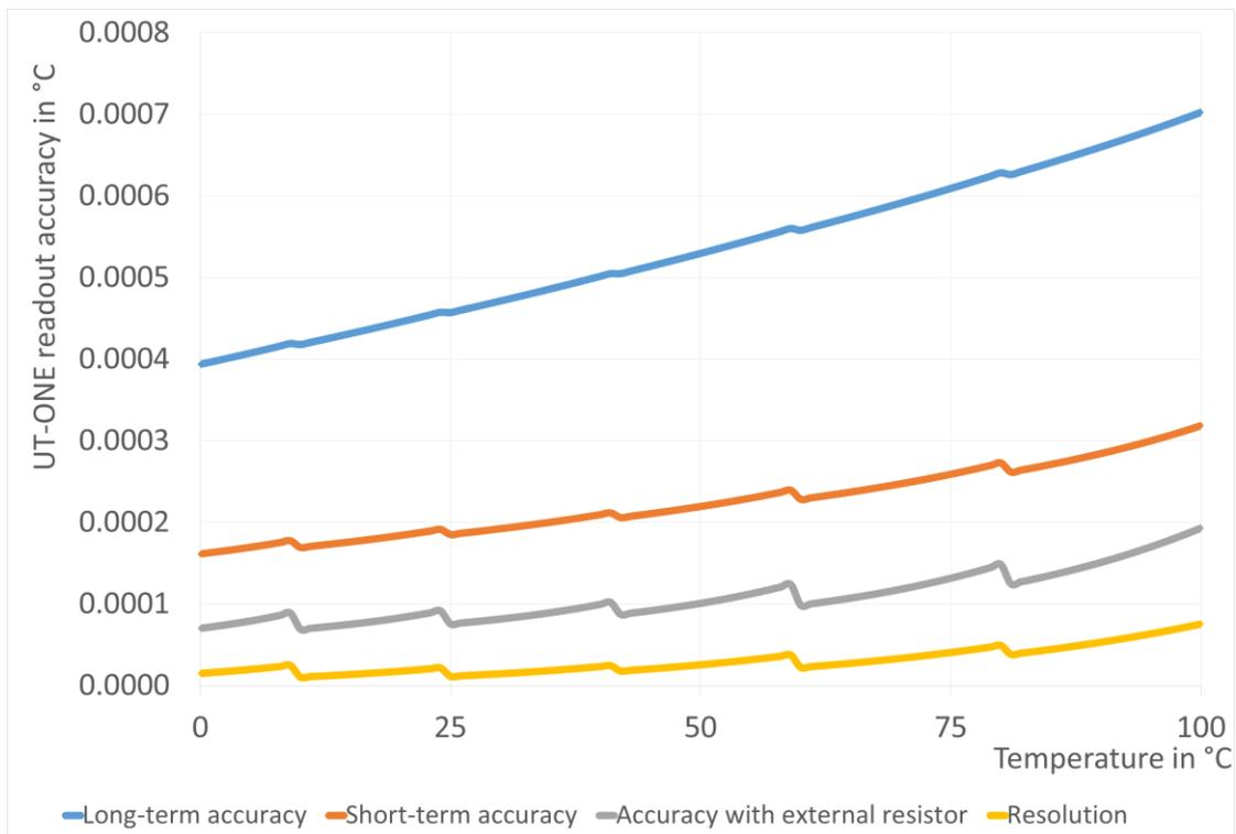
**Figure 79: UT-ONE accuracy specification for 10K3A thermistor probe**
