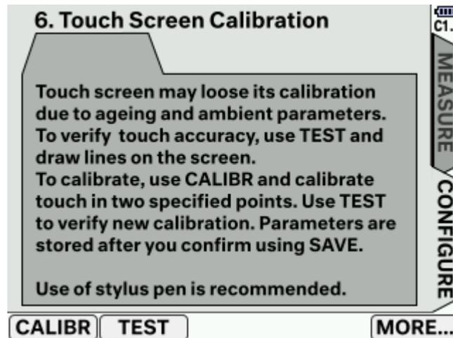
*Figure 32: Touch screen calibration window*
