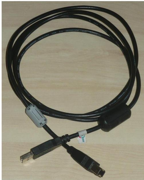
*Figure 52: USB cable with two ferrite cores*
