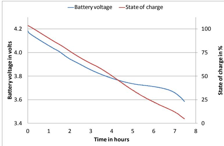
**Figure 54: Typical discharging characteristics of standard LiPo battery**
