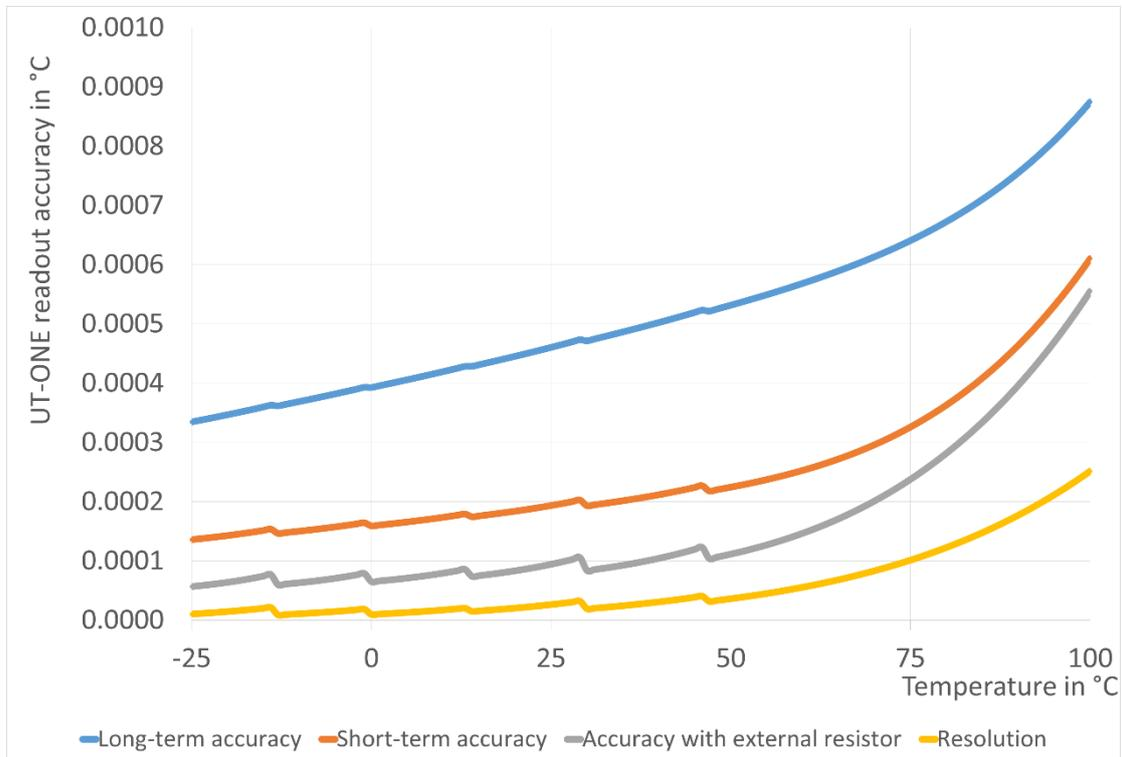
**Figure 77: UT-ONE accuracy specification for 3K3A thermistor probe**
