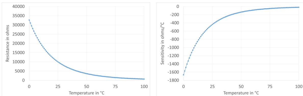
**Figure 80: Resistance and sensitivity characteristic for 10K3A thermistor probe**
