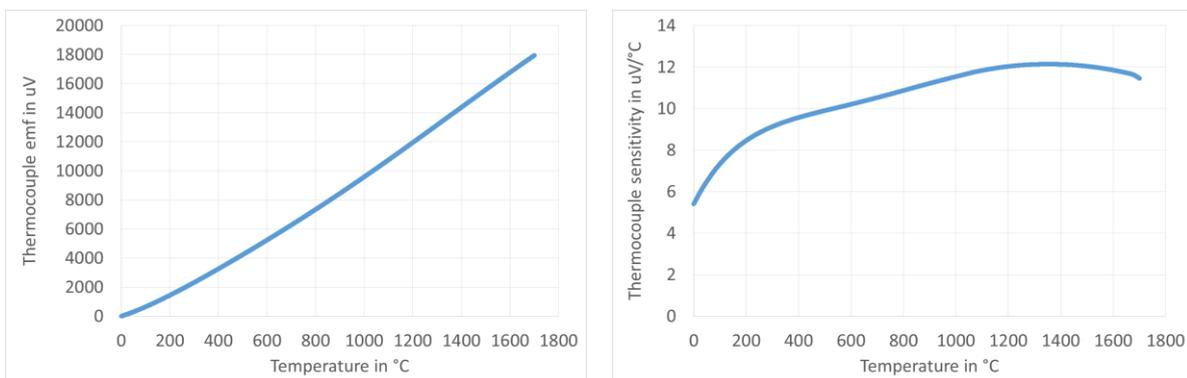
**Figure 84: Emf and sensitivity characteristic for type S thermocouple probe**
