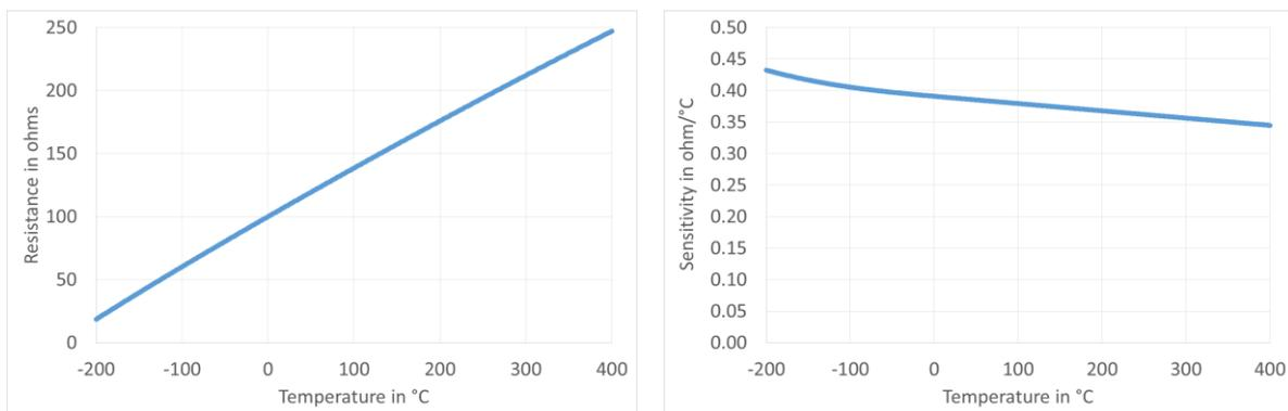
**Figure 74: Resistance and sensitivity characteristic for Pt-100 probe**
