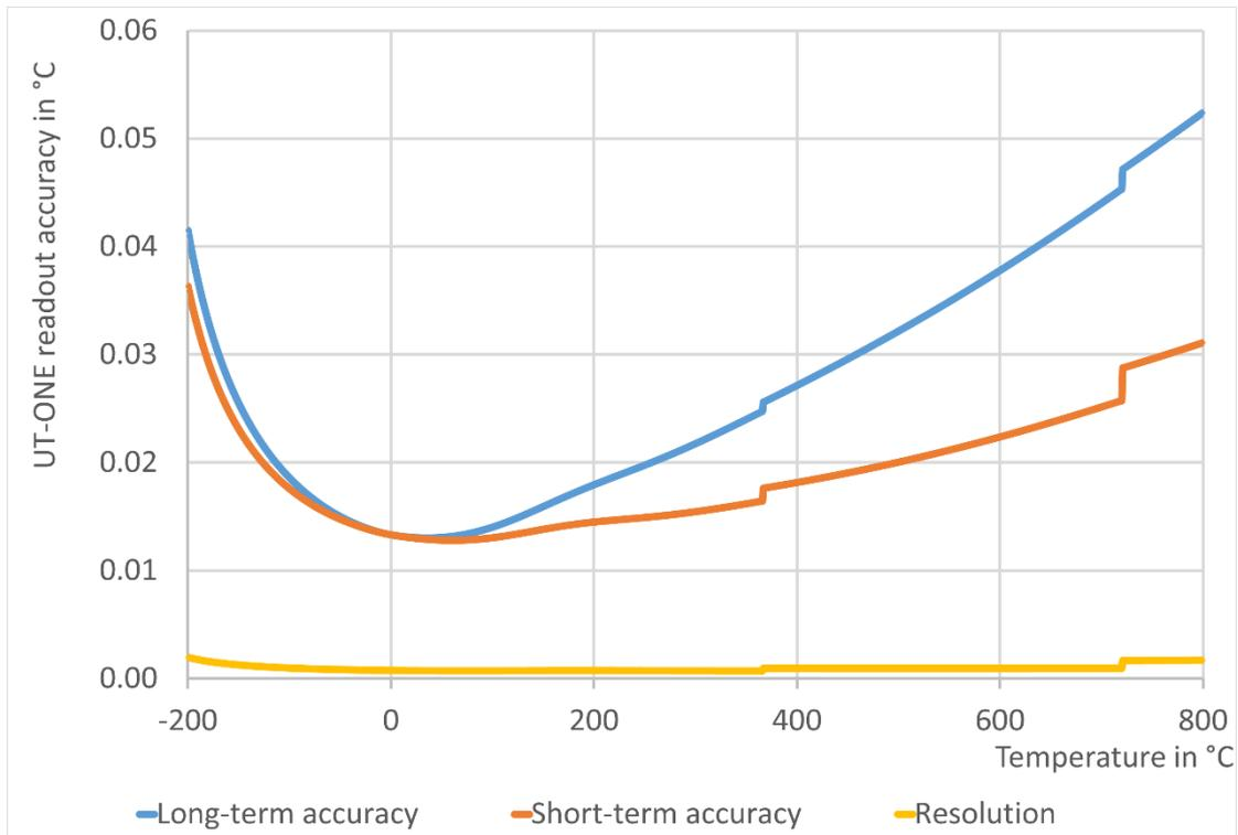
**Figure 81: UT-ONE accuracy specification for type K thermocouple probe**
