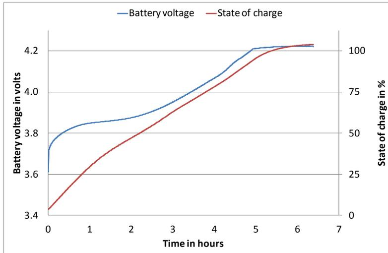
**Figure 55: Typical charging characteristics of standard LiPo battery**
