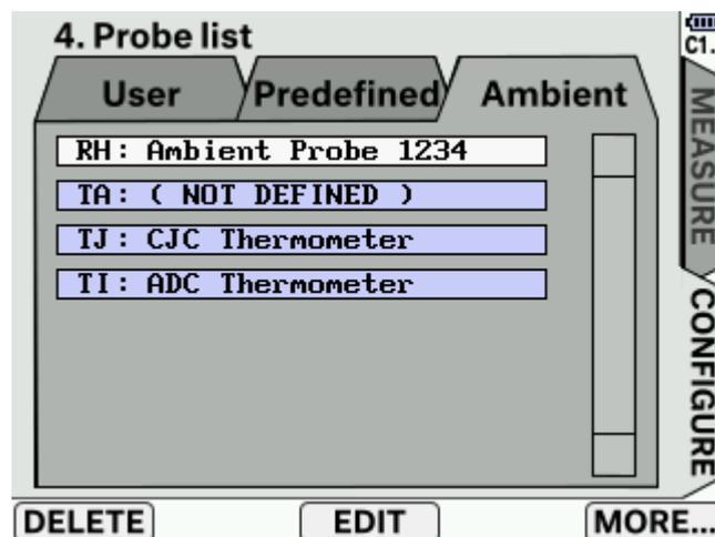
Figure 26: Ambient probe list
