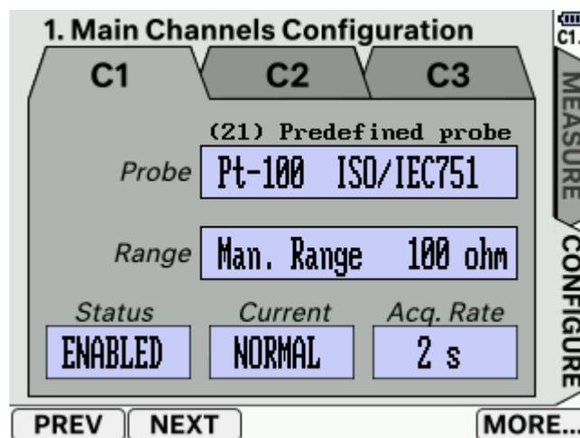
Figure 18: Main Channels Configuration
