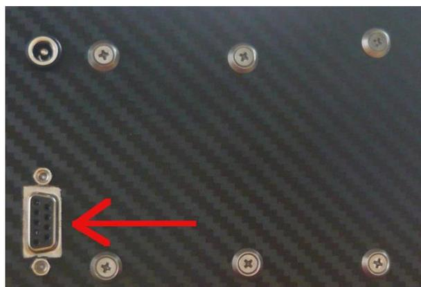
*Figure 48: RS232 connector on the back-side of UT-ONE*
