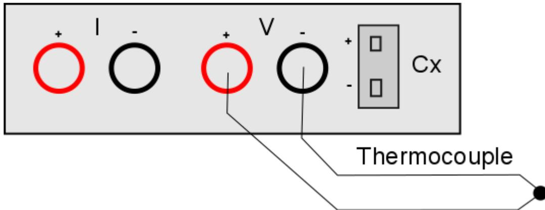
*Figure 7: Thermocouple connection using the voltage connectors*
