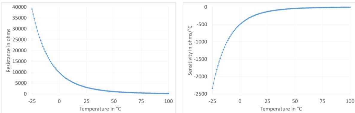
**Figure 78: Resistance and sensitivity characteristic for 3K3A thermistor probe**
