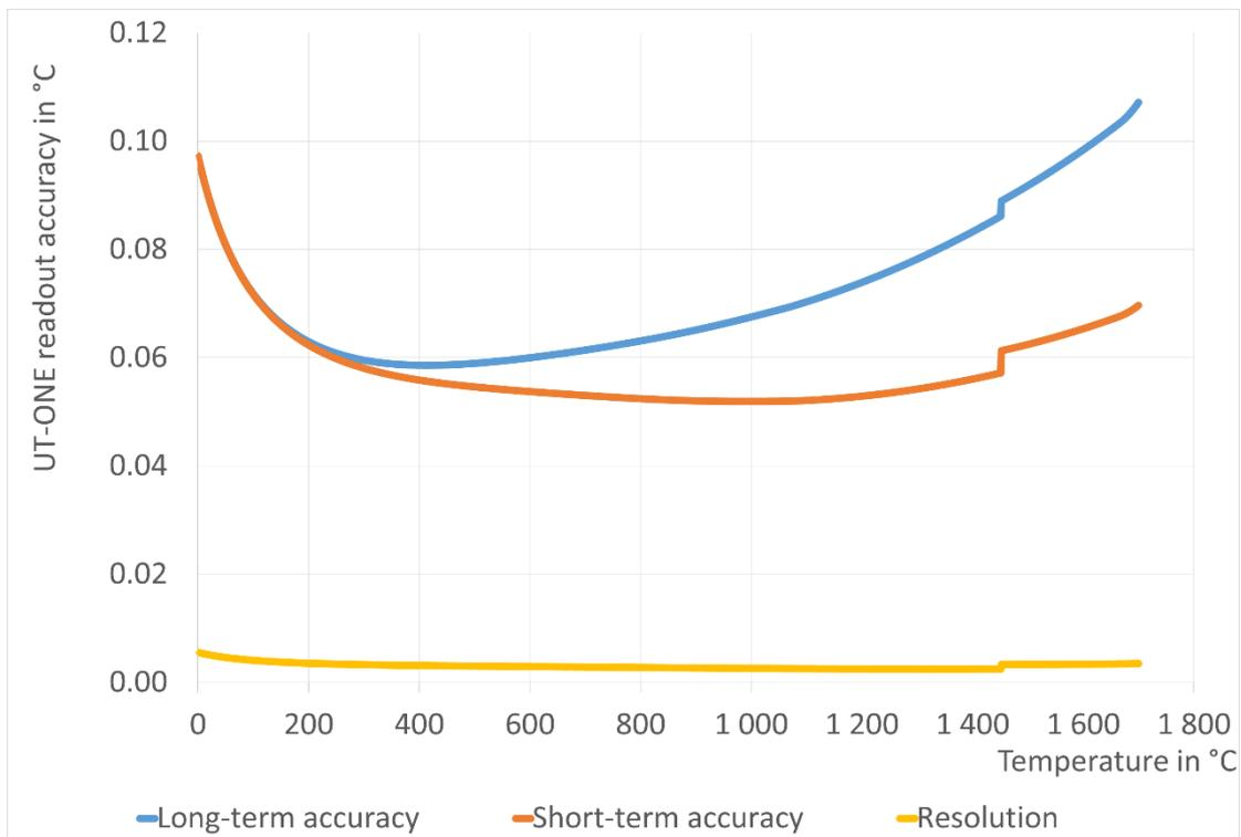
**Figure 83: UT-ONE accuracy specification for type S thermocouple probe**
