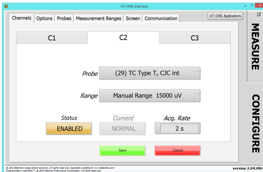
**Figure 60: UT-ONE Interface channel configuration view**
