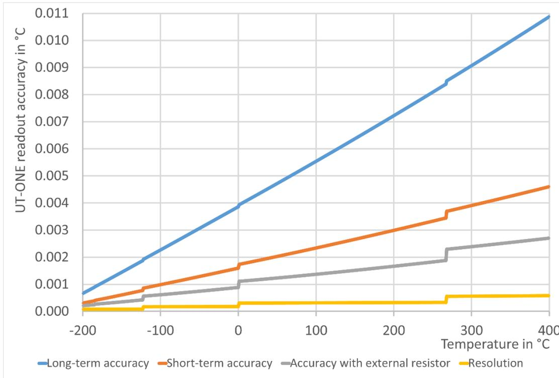
**Figure 73: UT-ONE accuracy specification for Pt-100 probe**
