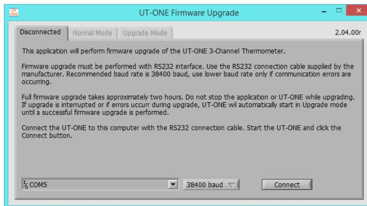
**Figure 69: UT-ONE Firmware Upgrade**
