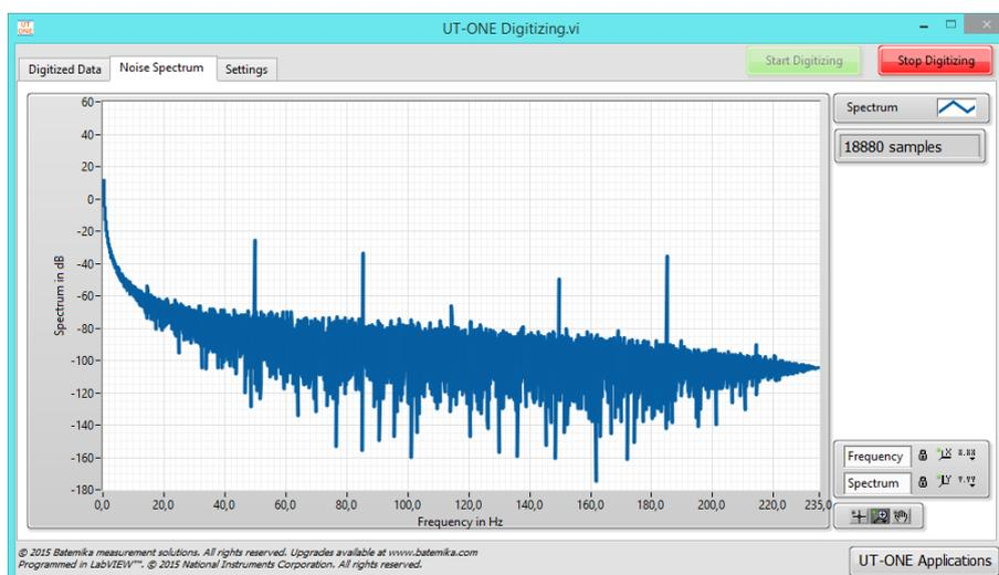
**Figure 67: Noise spectrum with considerable 50 Hz interference**
