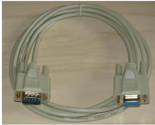
*Figure 49: RS232 connection cable*
