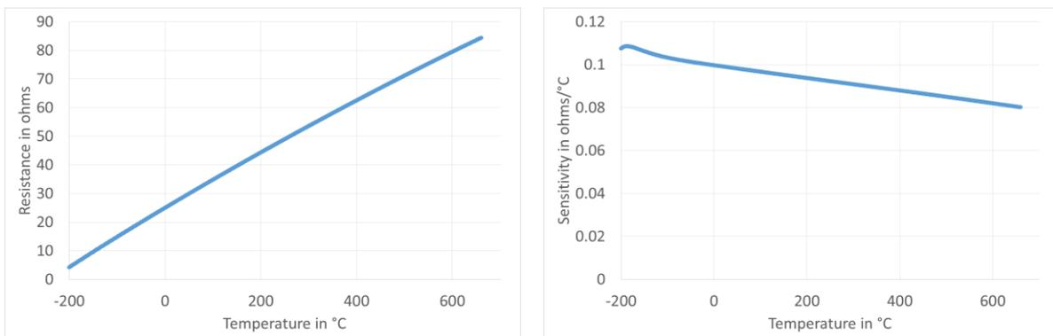
**Figure 76: Resistance and sensitivity characteristic for Pt-25 probe**
