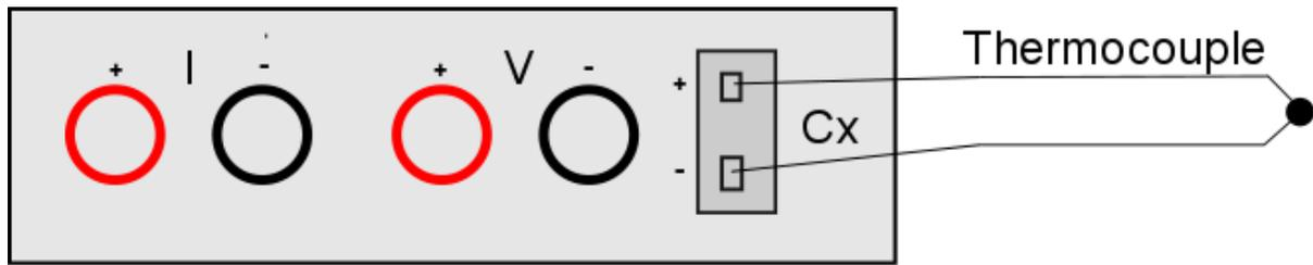
*Figure 6: Thermocouple connection using the thermocouple connector*
