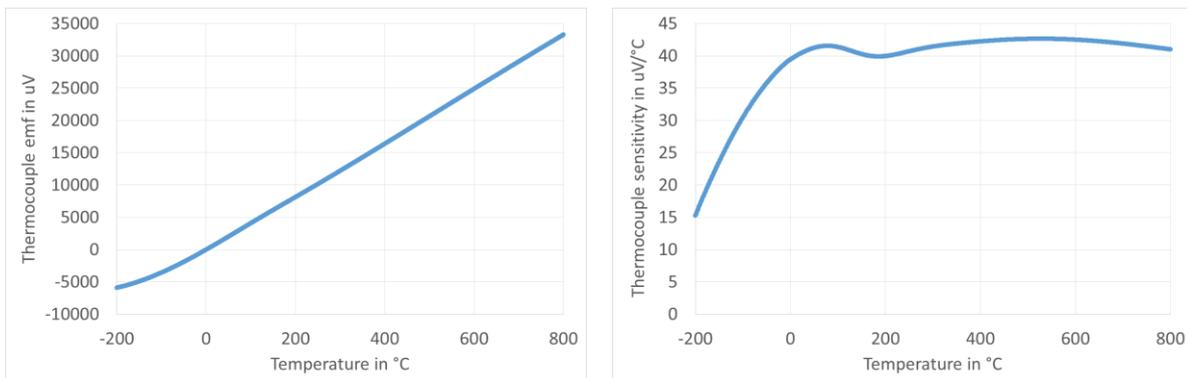
**Figure 82: Emf and sensitivity characteristic for type K thermocouple probe**
