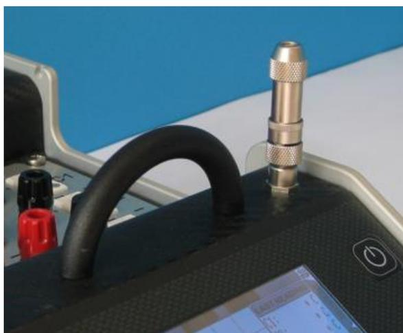
*Figure 9: Direct connection of ambient probe*
