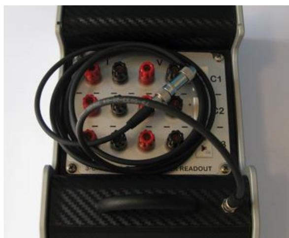
*Figure 10: Connection of ambient probe with 2 m extension cable*
