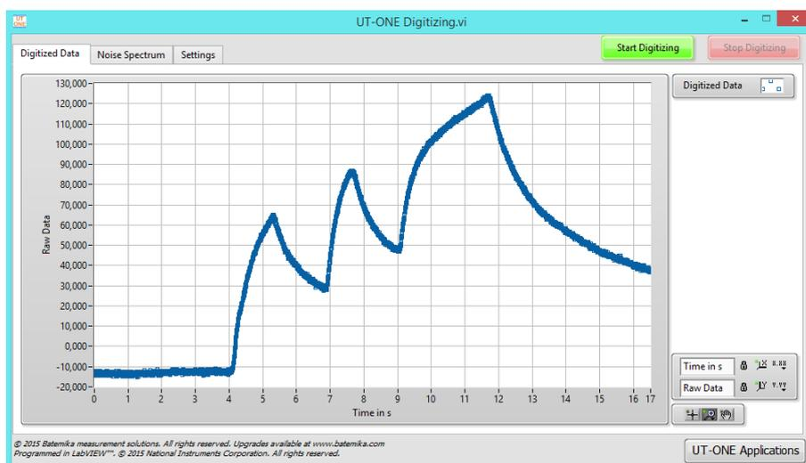
**Figure 66: Observing of fast transients in digitizing mode**
