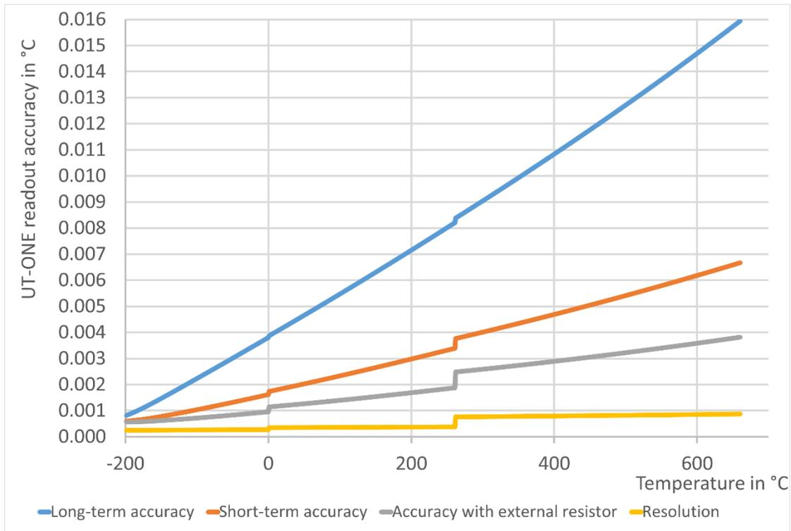
**Figure 75: UT-ONE accuracy specification for Pt-25 probe**
