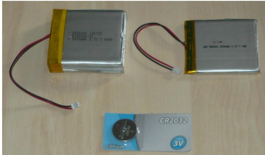
*Figure 53: UT-ONE batteries: extended or standard LiPo battery and button Li-ion battery*
