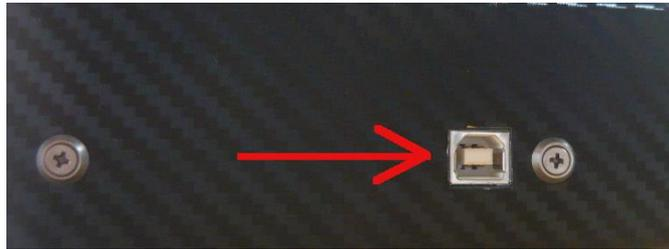
*Figure 51: USB connector on the front side of UT-ONE*
