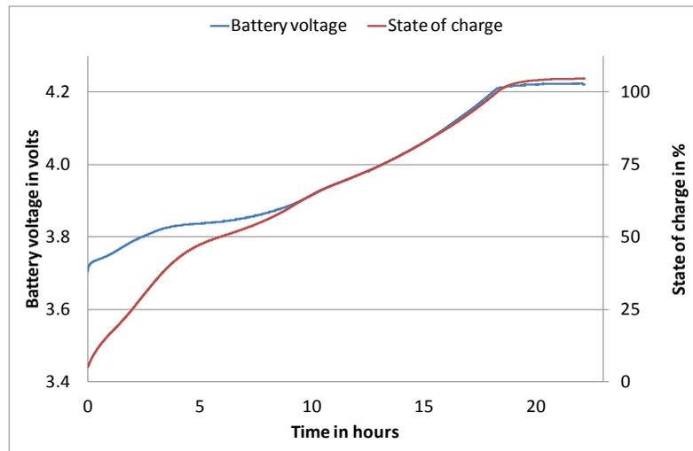
*Figure 57: Typical charging characteristics of extended LiPo battery*
