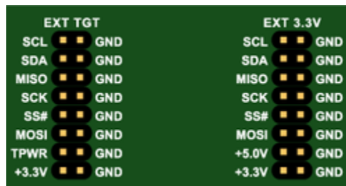
Figure 6 : The External Connectors provide the developer with a quick and easy way to interface or monitor any or all of the Level Shifter Board signals on either the Adapter/ Analyzer side or the target side.
