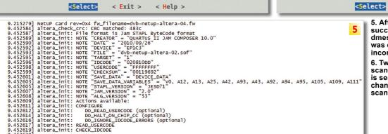
5. After compiling the kernel successfully, you should use dmesq to check if the card was correctly recognized and incorporated into the system
