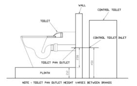
Remove the packing from the Control Toilet Unit. Locate the unit level ensuring toilet will drain to unit.
