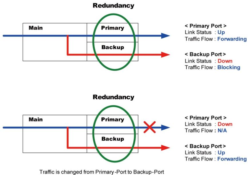
**Figure 2-5:** Redundancy Behavior Topology
