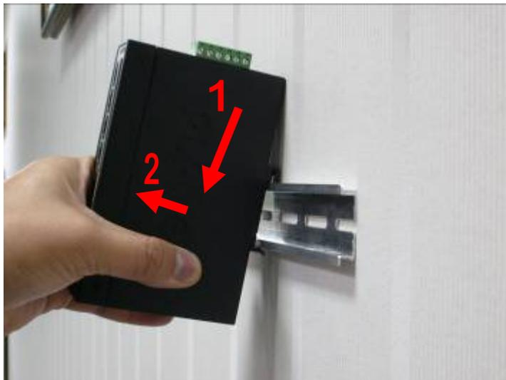
**Step 5:** Lightly pull out the bottom of the DIN-Rail from the track to remove.
