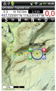
The info bar shows the total length of the path in the black field in the selected units. At the position marker you find the bearing, distance and slope from the previous point (see above).
