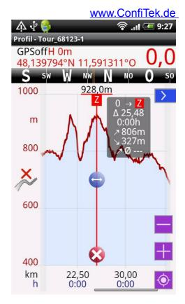
In the profile screen you can place the target marker (Z) and additionally a start marker (S). Read the exact height of this point at the top of the marker. Also you find tour data next to the target marker which is calculated from the beginning or from the start marker.
