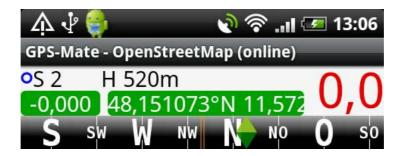
In the general settings you can choose the 'compass function' to either use a built-in electronic compass or the GPS. Please note that the GPS only updates the direction when you move.
