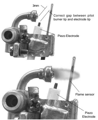
Fig. 13 - Characteristic Pilot Flame
