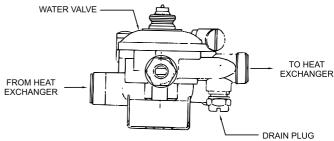
Fig. 0 - Water heater drain plug
