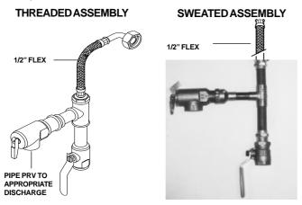
Fig. 8 - Plumbing connections for the Aquastar 125FX
