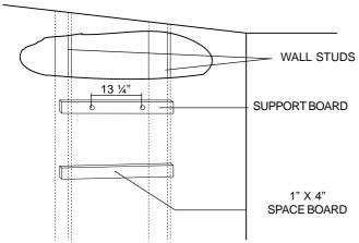
Fig. 2 - Mounting the Heater
