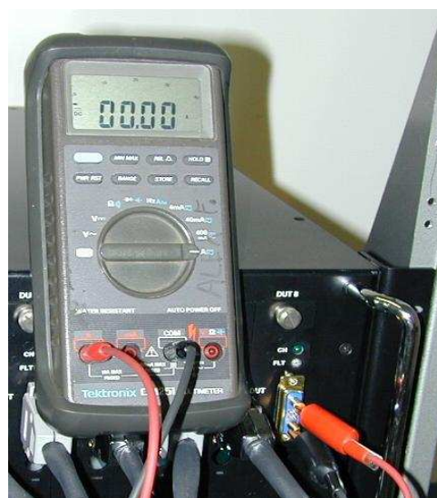
Current Meter Attached to Drain Force and Source Force
