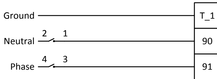
Figure 5.7. Wiring diagram of the power supply.
